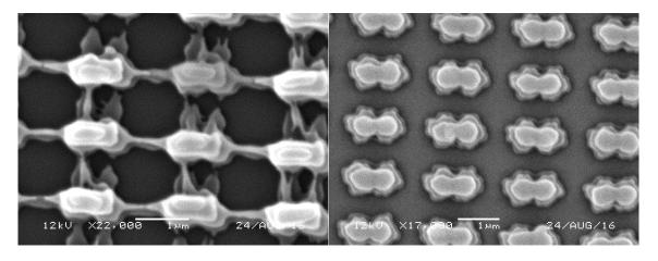
The first iteration is seen on the left and the second on the right after adjusting the write speed.
