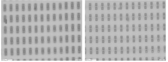
Identical frames at different depth of focus reveal that it is much easier to produce uniform arrays for characteristic features larger than  $\sim$ 700nm
