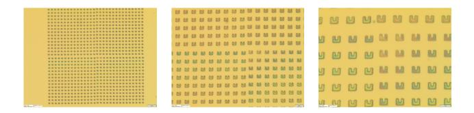
The ability to make large scale arrays of uniform microspheres is considered to be a disruptive technology for enhancing focal plane arrays in IR imaging systems (parametrically modulated type-III strained layer superlattice photodetectors).
