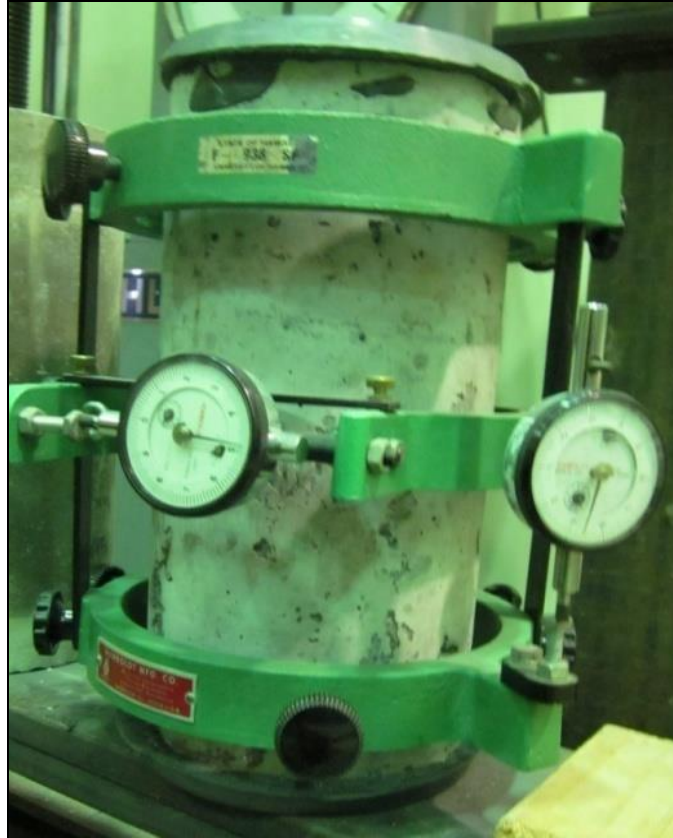
Figure 15. Compressometer-extensometer used to measure the Poisson's ratio in the 6-inch-diameter geopolymer specimens
