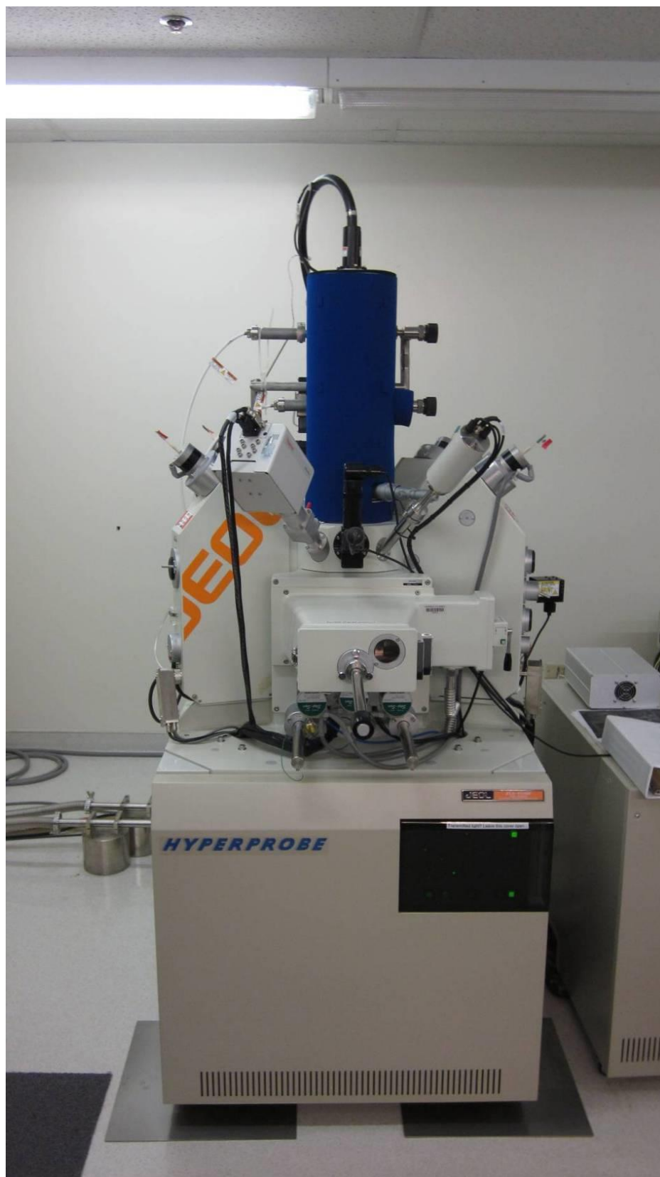
Figure 22. Electron Probe Microanalyzer used in the SEM with EDS analyses
