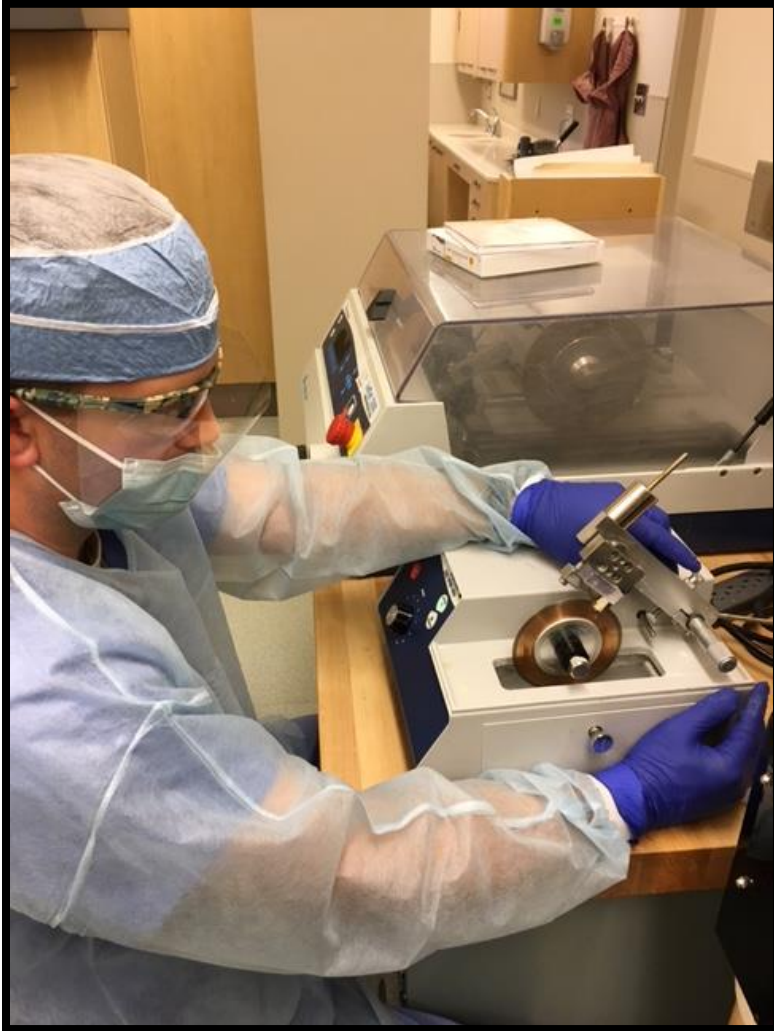
Figure 3. Specimen preparation on the Buehler IsoMet Low Speed Saw
