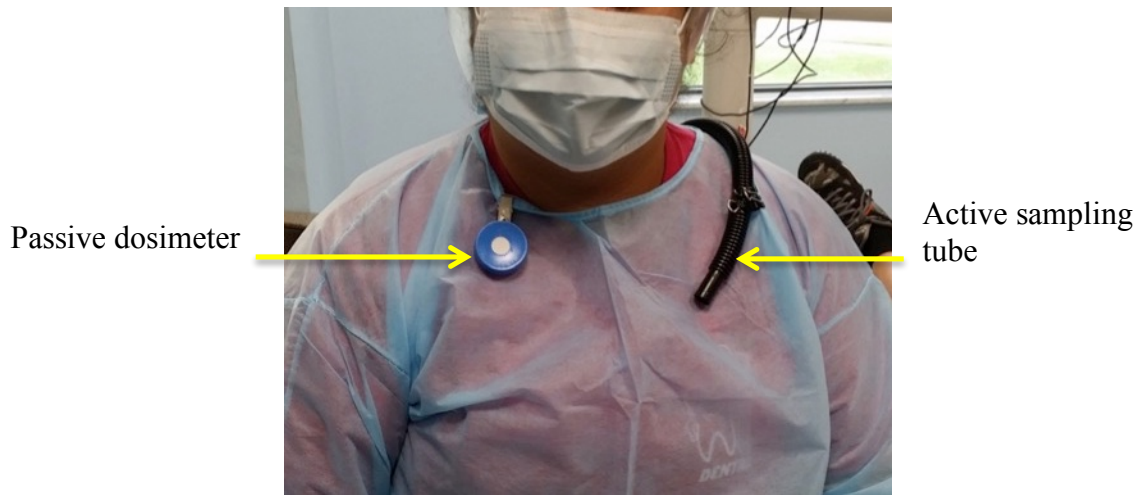
Figure 3: Active and passive sampling devices and how they were positioned during the sampling process.
