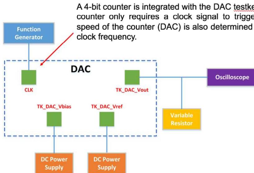
**Figure 20: The test setup for the DAC**
