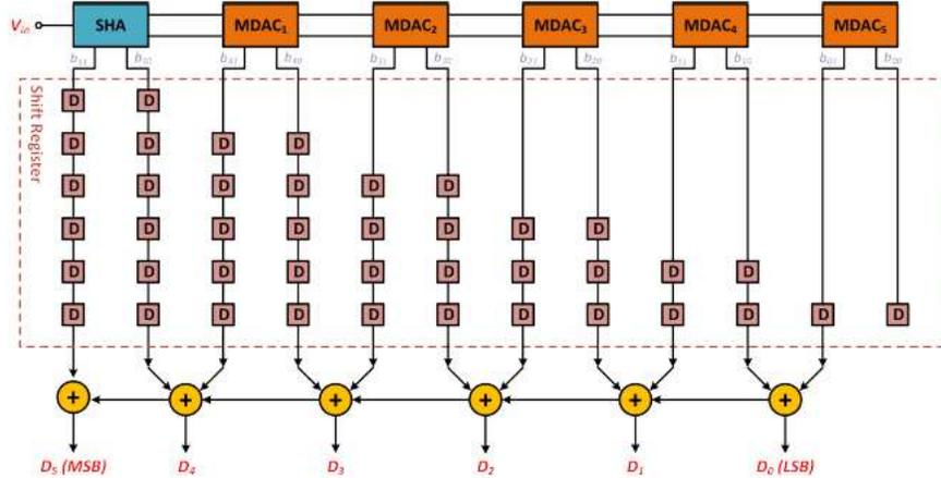
**Figure 15: Simplified schematic of redundancy algorithm logic circuit**
