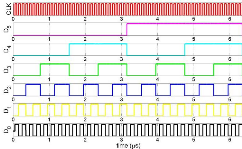
**Figure 6: Waveform of the 6-bit Synchronous Counter**
