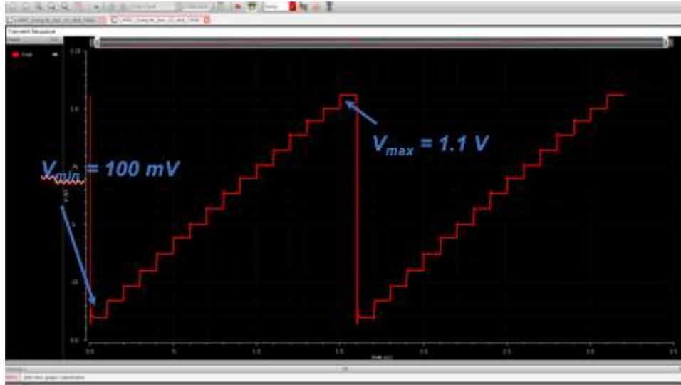
**Figure 10: The simulation results of the current-steering DAC**
