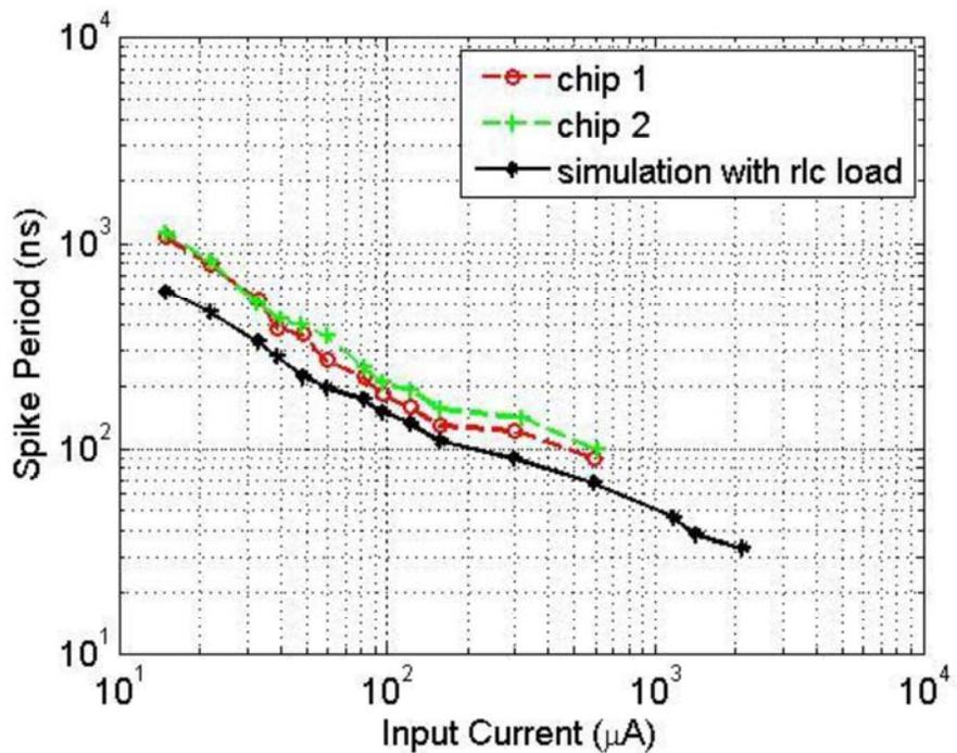
Figure 18: The measured spike period versus current
