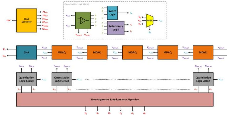
**Figure 13: Simplified schematic of 6-bit 1.5b/stage pipelined ADC**
