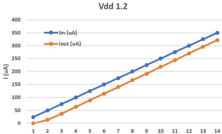
Figure 23: The TIA's input and output current
