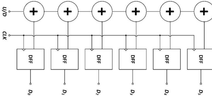
**Figure 5: The simplified schematic of 6-bit Synchronous Counter**
