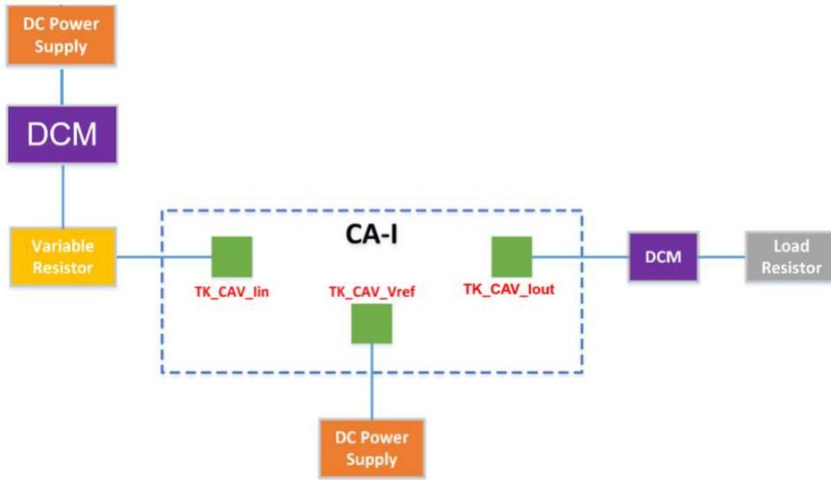
Figure 22: The test setup for the TIA
