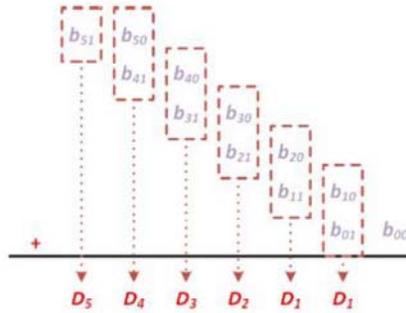
**Figure 16: Summation technique of 1.5 b/stage redundancy bit**
