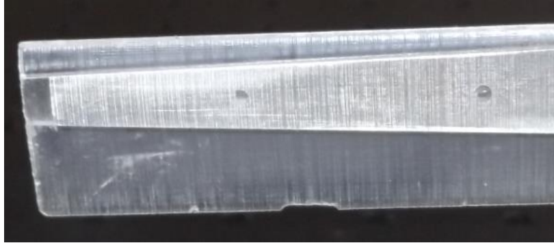
Fig. 5 Photo of canard blade with damaged trailing edge
