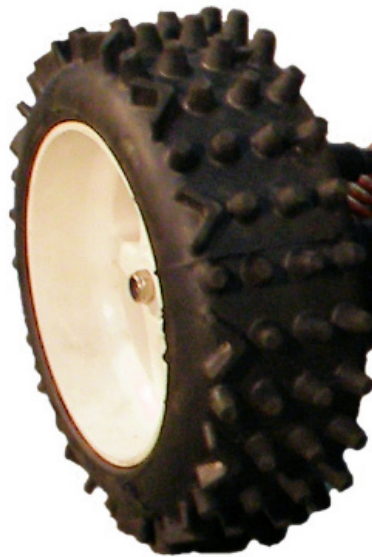
Figure E-13: Tire Pattern Problematic for Collision Detection.
