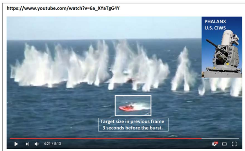
Figure 1. CIWS Phalanx Operating against Inflated Boat. Adapted from [5].
