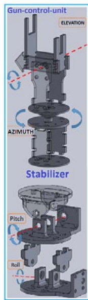
Figure 13. Prototype's Overall Design in SolidWorks Software
