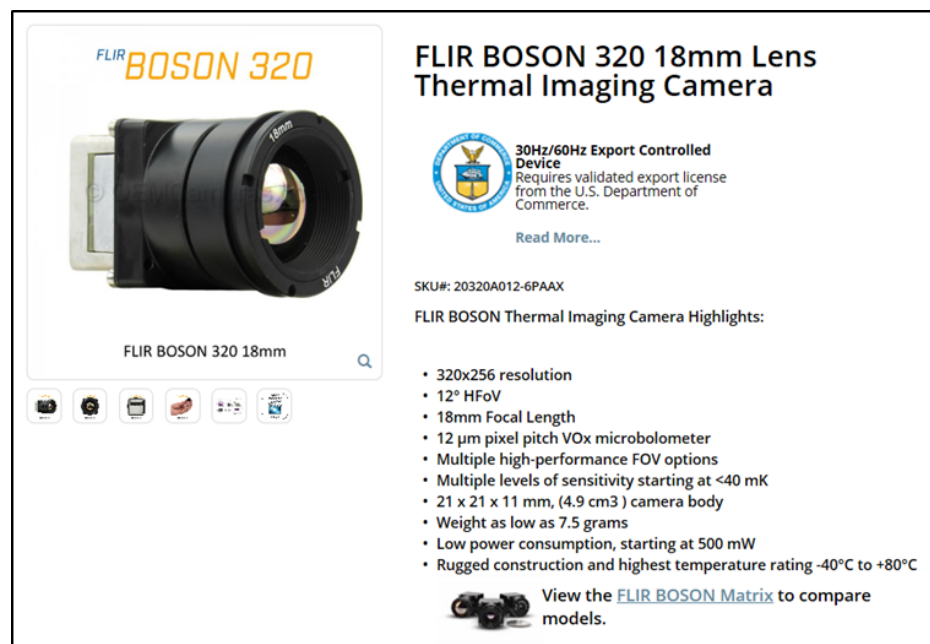
Figure 16. FLIR BOSON Camera Specifications. Source: [37].
