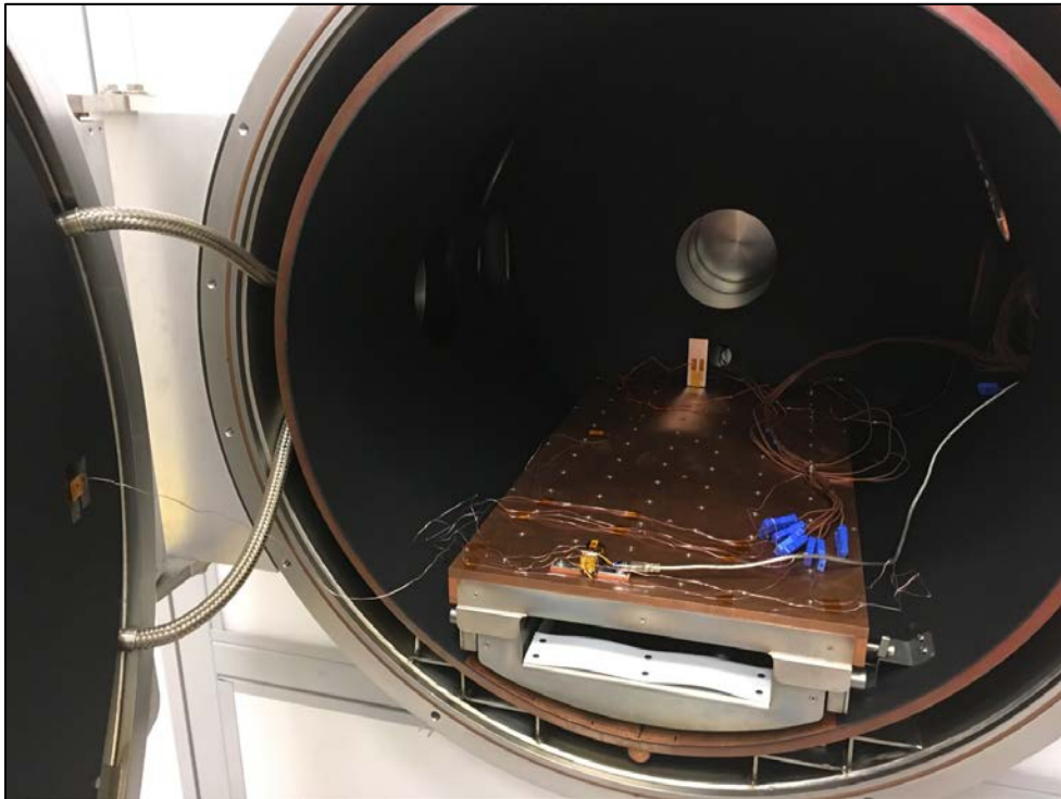
Figure 45. Second TVAC Test Setup of TIC EDU and IR Source
