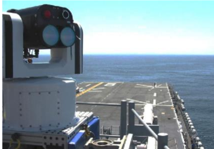
Figure 25. FSO Terminal on USS Bonhomme Richard . Source: [9].
