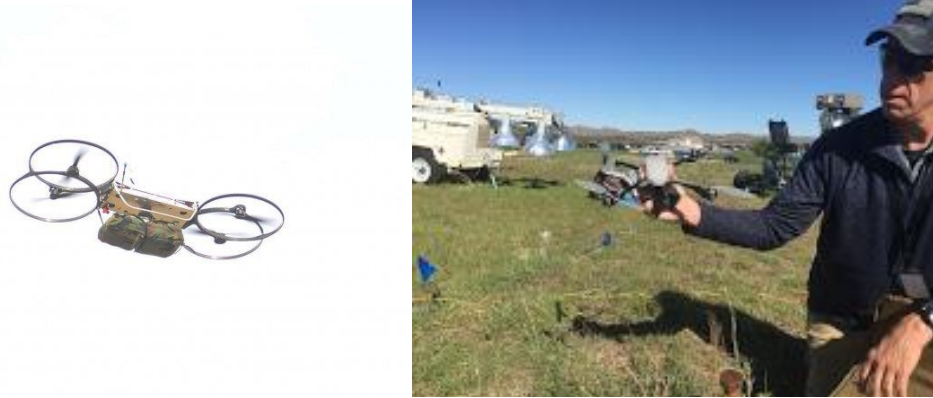
Fig. 3 Photographs of the two UAVs imaged during the test. The UAV on the left is a prototype OEM vehicle (often termed a JTARV), which is approximately 1 m in length. The smaller UAV on the right is a commercially available drone called InstantEye, which measures approximately 12 inches in length.
