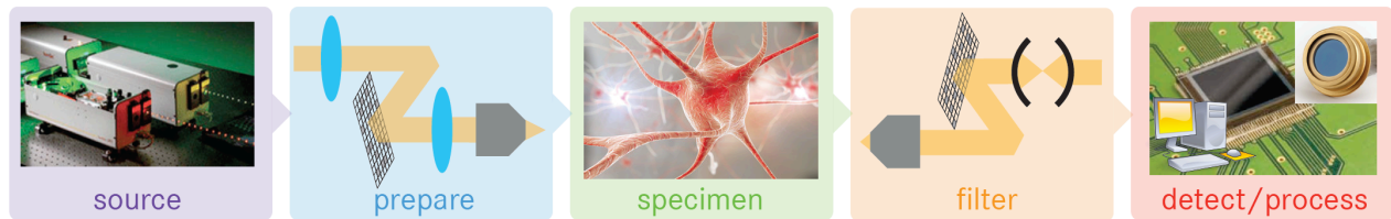
Figure 2: Elements of an optical measurement
