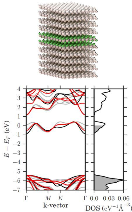
Fig.9 A low loss material T-AlCl<sub>2</sub> (top) crystalline layered structure (bottom) Band structure
