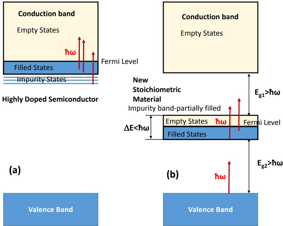
**Fig.8** (a) Highly doped semiconductor with strong absorption. (b) Novel stoichiometric material that exhibits no absorption in a range of frequencies that are too high for the intraband absorption and too low for the interband absorption.
