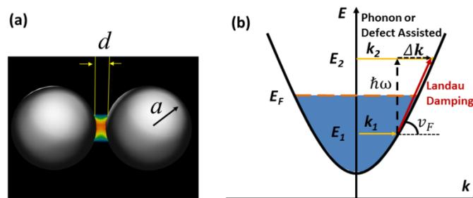
Fig. 4. (a) Illustration of the SPP field concentration in plasmonic dimer and (b) origin of Landau Damping – direct transition between two states with different wave-vectors  $k_1$  and  $k_2$ .
