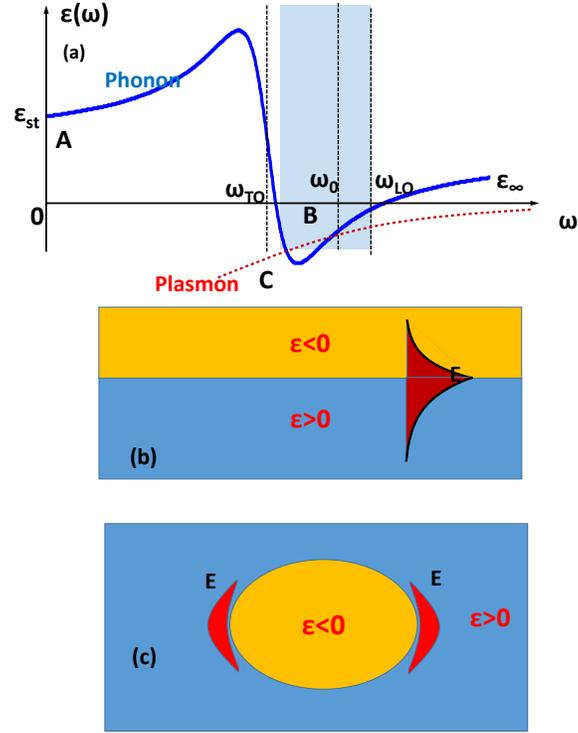
Fig. 2 (a) Dispersion of phonons and plasmons. (b) Propagating SphP; (c) Localized SPhP
