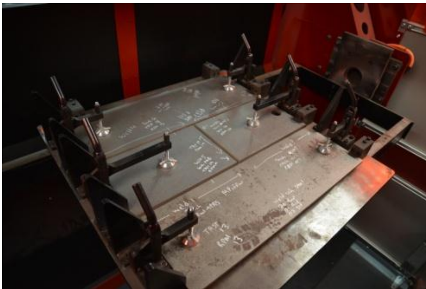
Figure 6. H-Plate Clamped and Ready for Welding.
