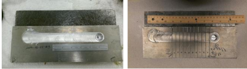
Figure 8. Representative SFSW weld between AA6061 and RHA (left). Welds sectioned via water jet as shown right, were used for testing and characterization.
