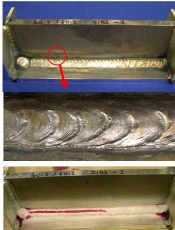
Figure 1. Aluminum Alloy 6013 + 6013 Welded with 5183 Filler Wire.
