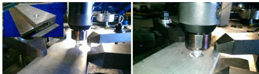
Figure 7. SFSW weld setup ready for joining (left) with inset Configuration as shown in the upper left inset picture. A hole is pre-drilled in the Al plate (right) prior to welding.
