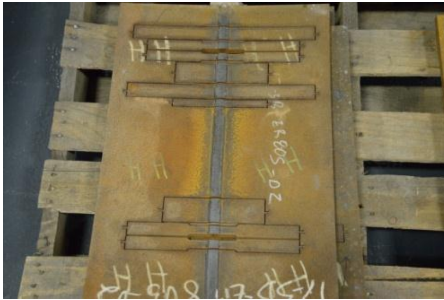
Figure 9. I-Plate Marked Samples for Standardized Weld Characterization Tests.
