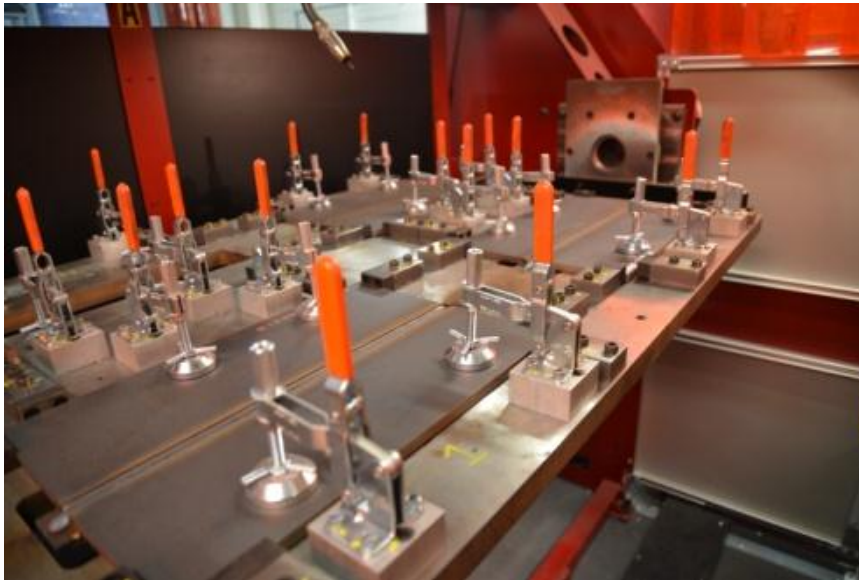
Figure 4. Fixture for Robotic Welding of I-Plate
