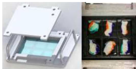
Figure 4. Specimen tray. Render of the design files used for the interchangeable specimen tray (left) and the system as fabricated and loaded with 6 inked, bread loaf sectioned breast specimens (right). The tray incorporates a lid with fill port as well as inset dividers that can be used to separate multiple small specimens.
