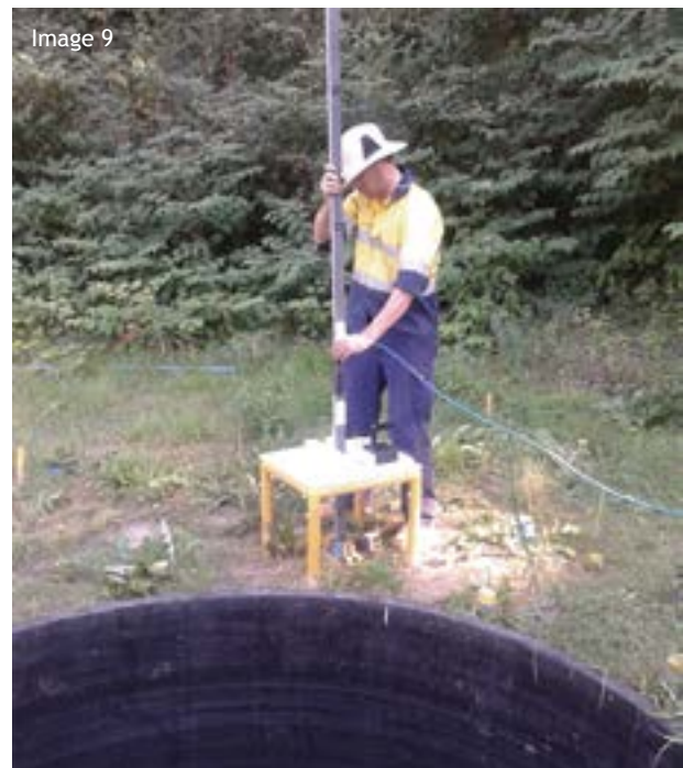
Images 8 and 9. Data collection at a borehole test pit. A 3 m deep test pit is used to collect measurements of ordnance that are then added to a reference library of target polarizabilities. The test pit is also used to collect QC measurements that verify classification processing.
