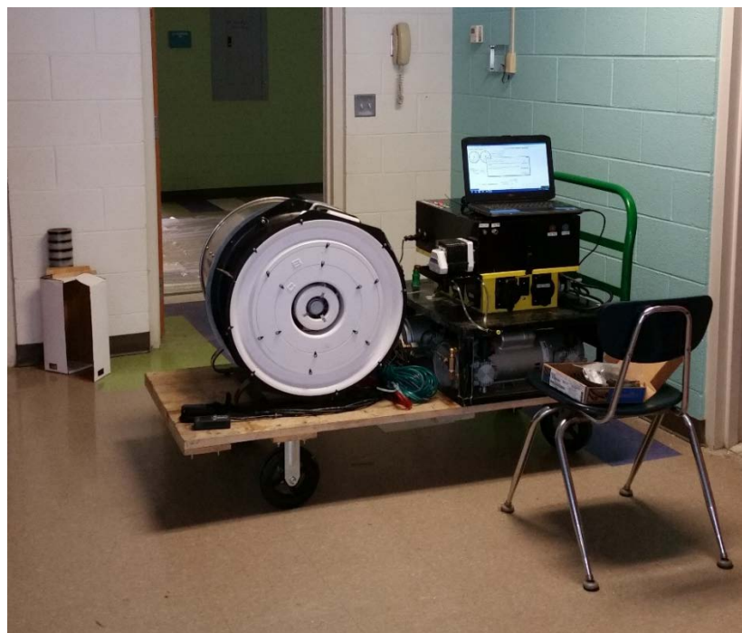
Figure 14: Photo of aerosol sealing equipment setup
