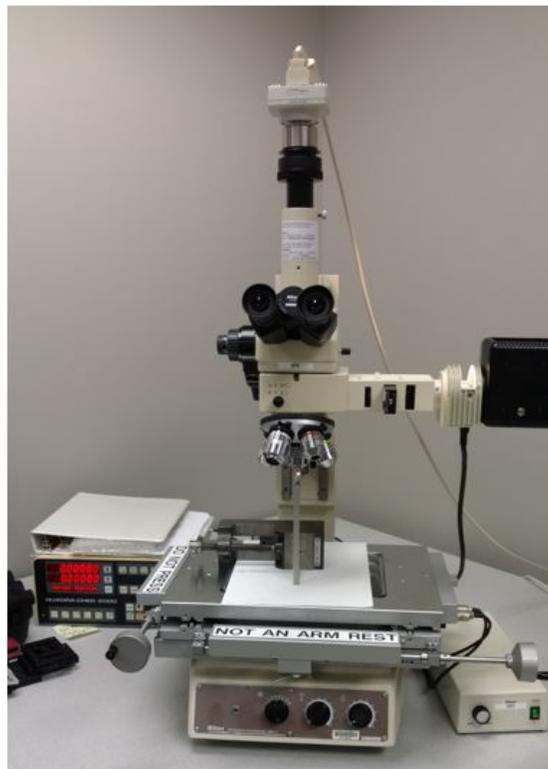
Figure 3.28. Optical microscope with integrated XY measuring table.
