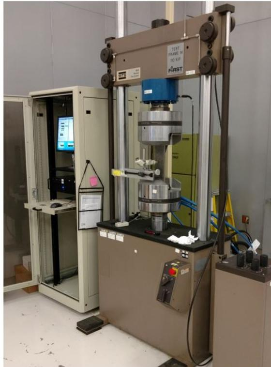
Figure 3.6. MTS Load cell with traveling microscope attached
