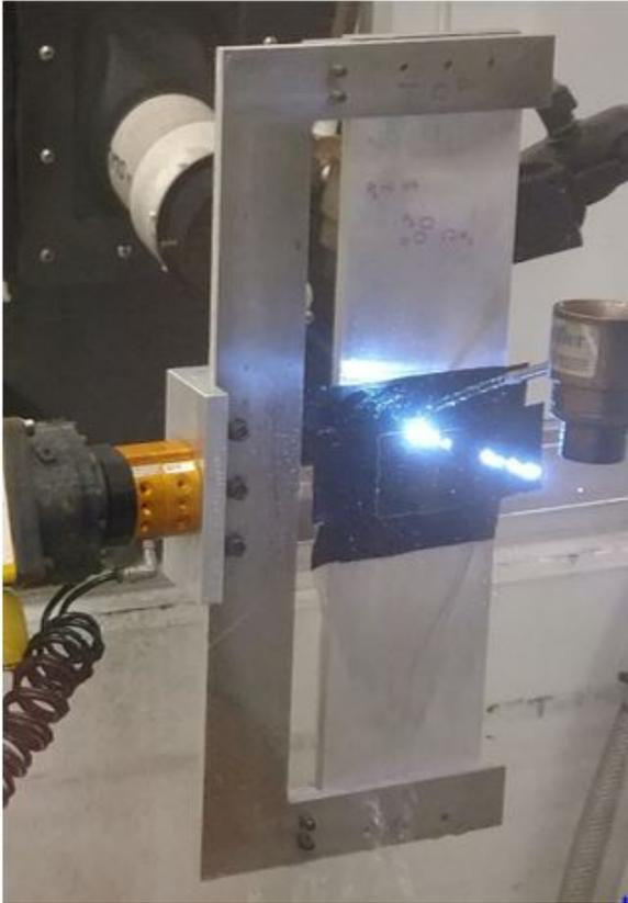
**Figure 3.14. Circle Spot Laser Peening Fixture**
