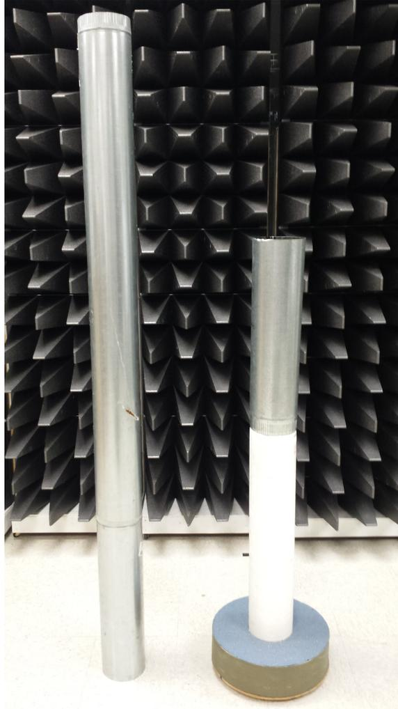
Figure 7. Metal cylinders used as radar targets
