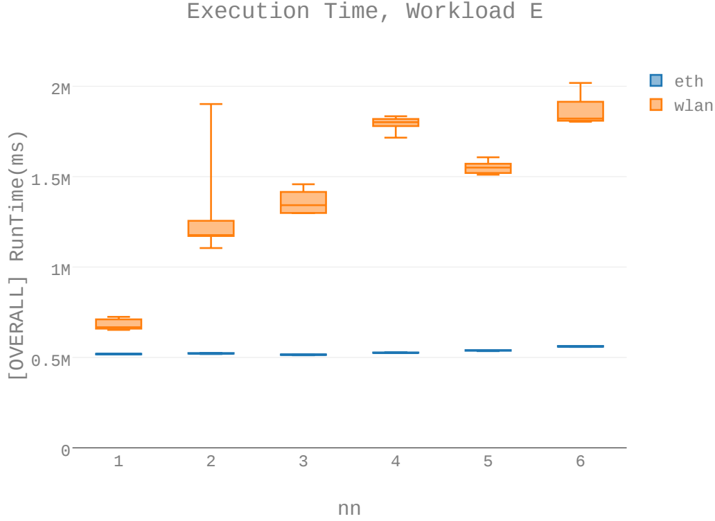
Figure 21. For 21 trials of 10,000 operations each of Workload E, this graph represents the execution time of a wired Ethernet cluster (eth) alongside the execution time of a wireless 802.11 cluster (wlan) with one exception. For Workload E on cluster size 6 on wireless local area network, erroneous results have been screened out, leaving 5 fully successful trials to be graphed, not 21.
