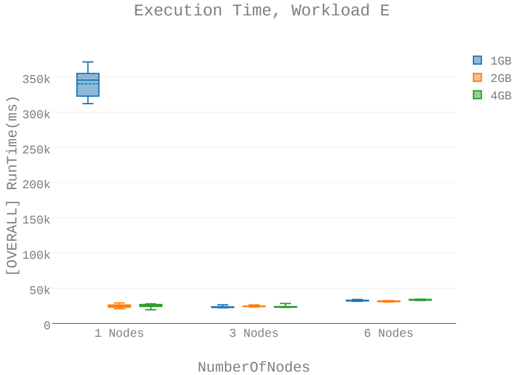
Figure 15. Variation in RAM over Workload E for the virtual machine clusters.
