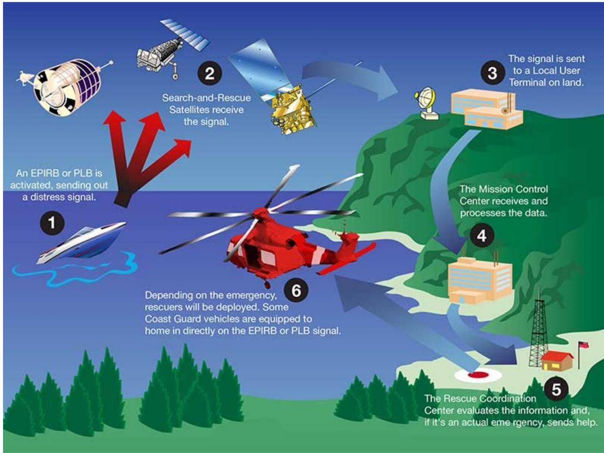
Figure 8. System overview of COSPAS-SARSAT system [4]
