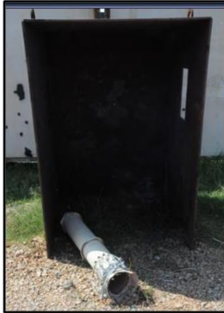
Figure 38 Container propelled into steel wall
