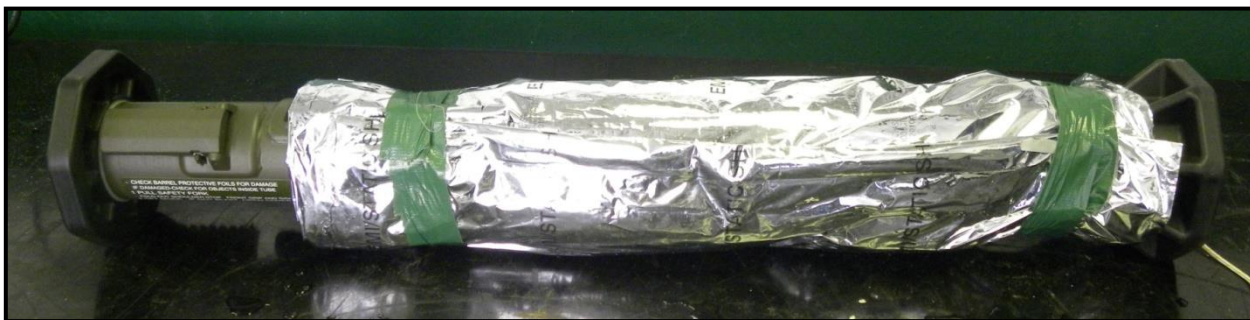
Figure 27 Blister liner enclosed with sealed foil/plastic barrier material
