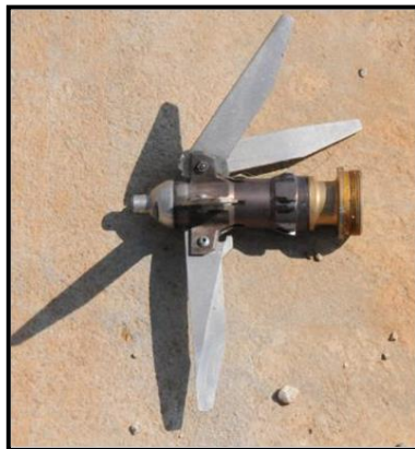
Figure 42 Recovered unarmed fuze and fin assembly (x-rayed)
