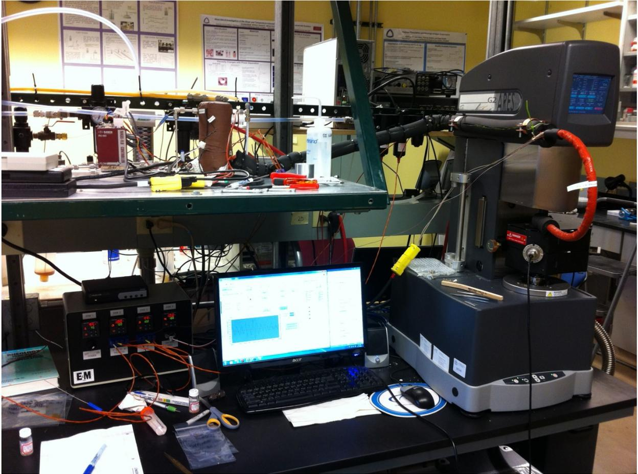
Figure 147: Humidity delivery system attached to ARES G-2 rheometer.
