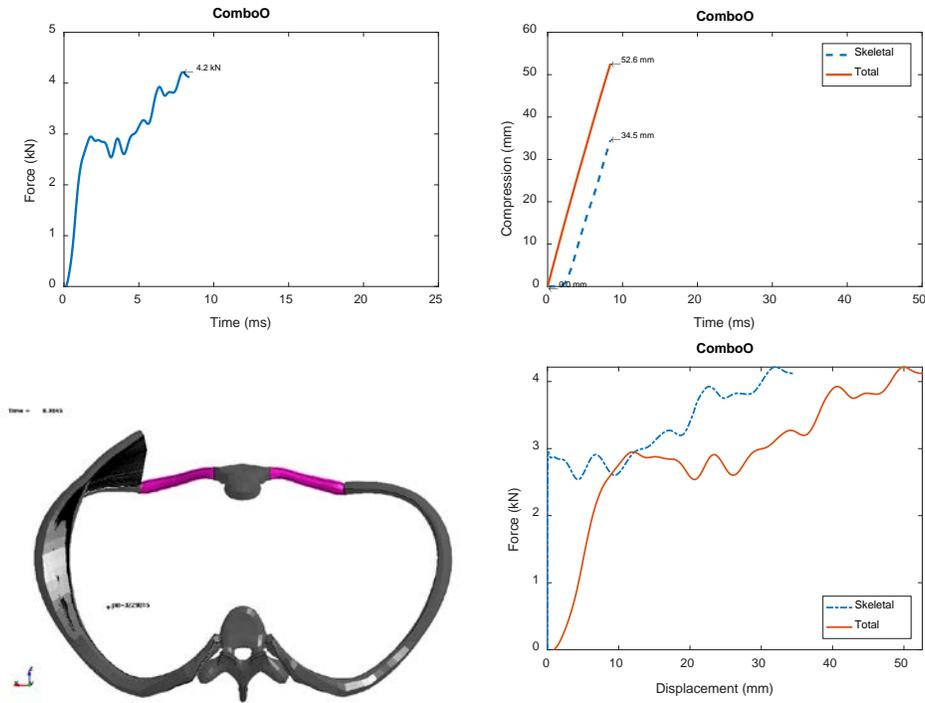
**Fig. 20 ComboO simulation results: force-time (upper left), compression-time (upper right), trace of fifth rib to maximum compression (bottom left), force-displacement (bottom right)**
