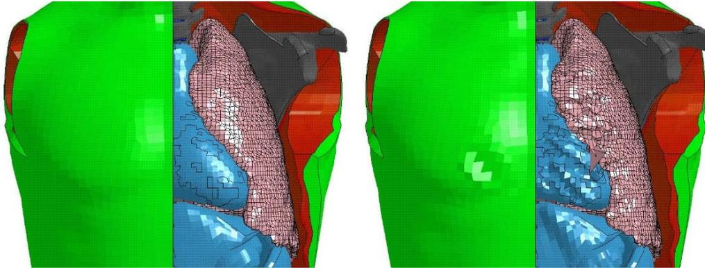
**Fig. 9** Foam simulation: left lung was distorted from original mesh (left) to unstable mesh at 4.4 ms (right) due to localized loading from the left ribs. Left ribs, clavicle, and sternum not shown to improve visibility of organs.
