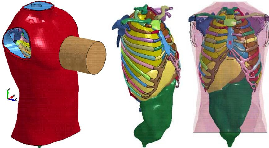
**Fig. 3** Full ARL torso model (left); model with flesh, impactor, and skin hidden (middle); frontal view with transparent impactor, flesh, and skin to show center of impact location (right). All colors randomly assigned to improve contrast.
