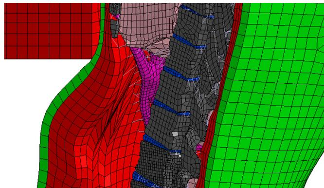
**Fig. 22 All simulation: sagittal plane view of the warped flesh elements from a behind-left oblique viewpoint. The liver, gallbladder, and intestines have been hidden to show the interior flesh surface.**
