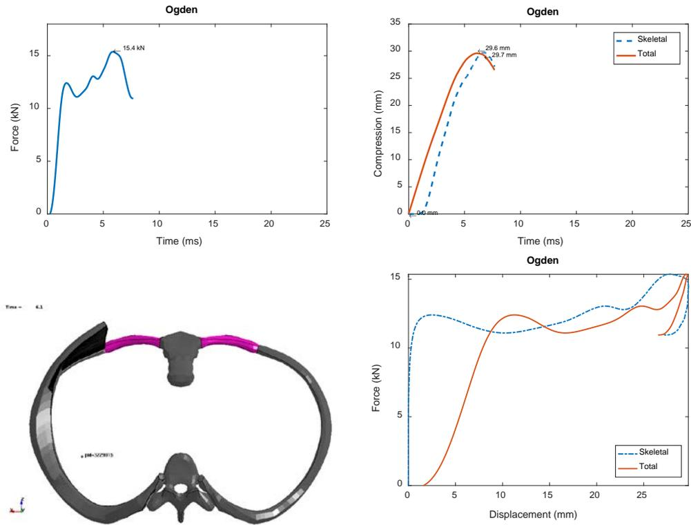
**Fig. 15** Ogden simulation results: force-time (upper left), compression-time (upper right), trace of fifth rib to maximum compression (bottom left), force-displacement (bottom right)
