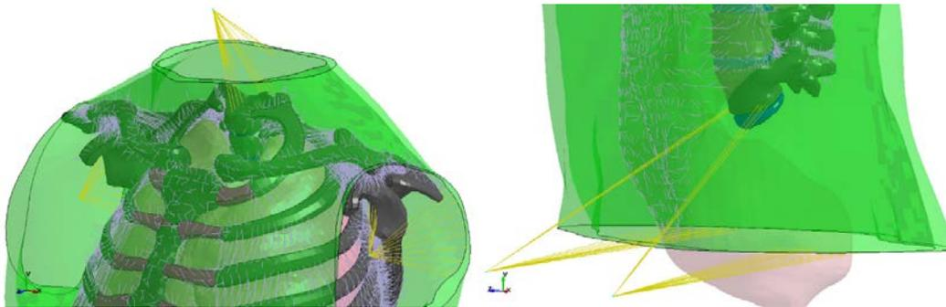
**Fig. 24 Stiffened ligaments, shown as orange lines, connect the point masses representing unmeshed head and arms to the neck and shoulders (left) and the lower abdomen and legs to the flesh and vertebrae above the hips (right)**
