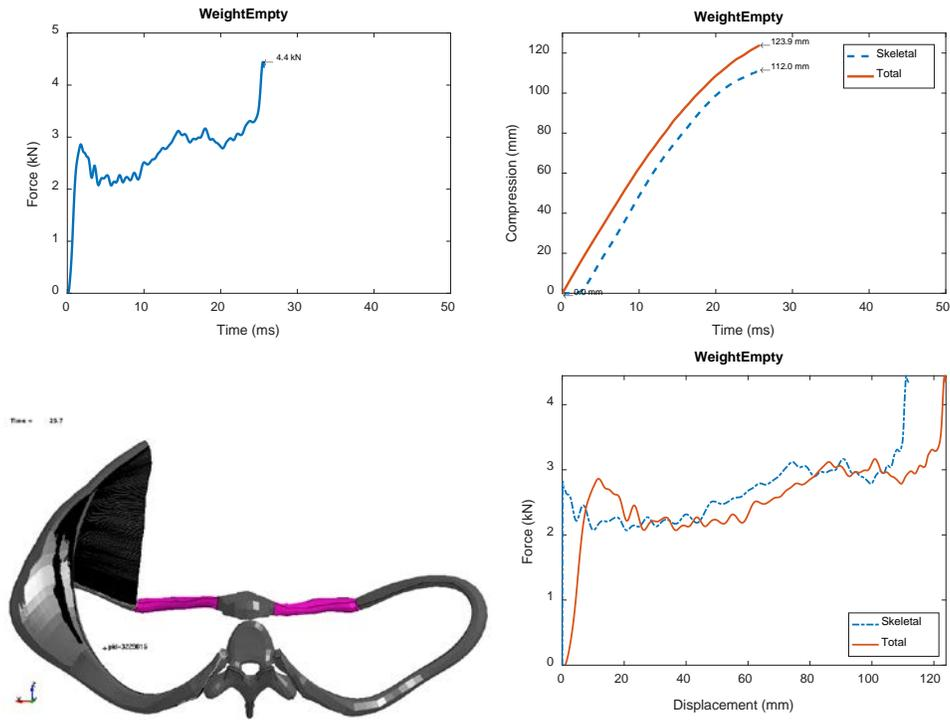
**Fig. 27** WeightEmpty simulation results: force-time (upper left), compression-time (upper right), trace of fifth rib to maximum compression (bottom left), force-displacement (bottom right)
