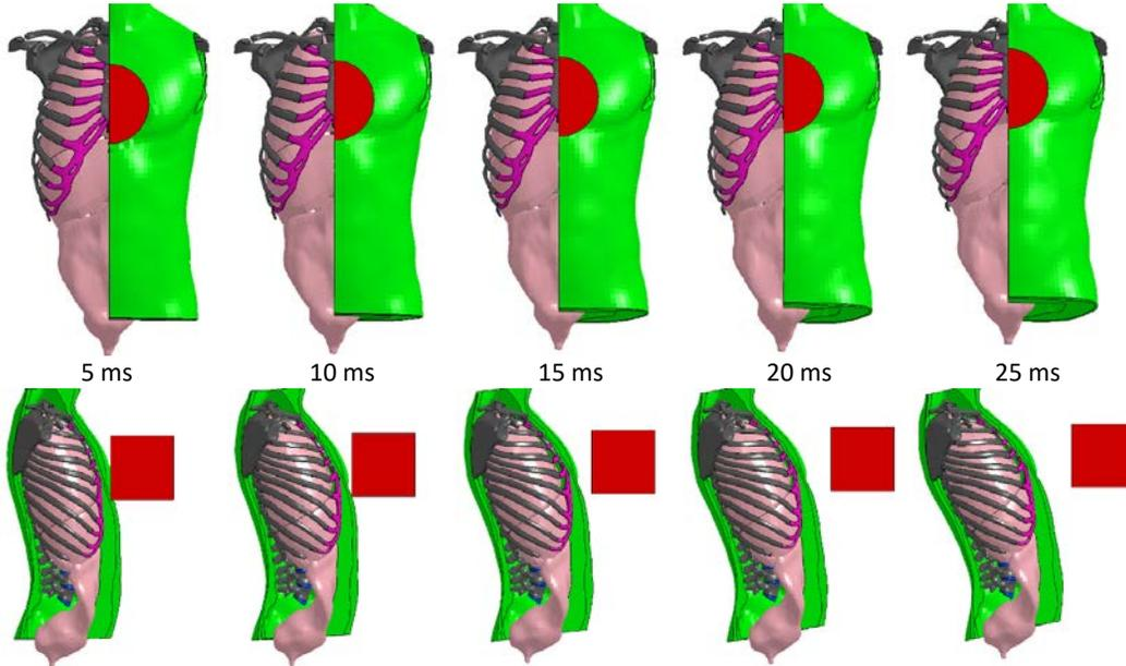
**Fig. 6** Original simulation chest response as seen from front (top) and side (bottom). Half of the flesh, skin, and impactor have been hidden to show the bone and organ response.
