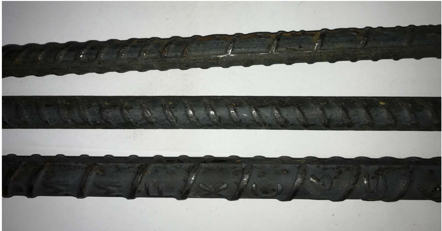
Figure 4. Samples of MMFX2 rebar installed at Bridge 9.
