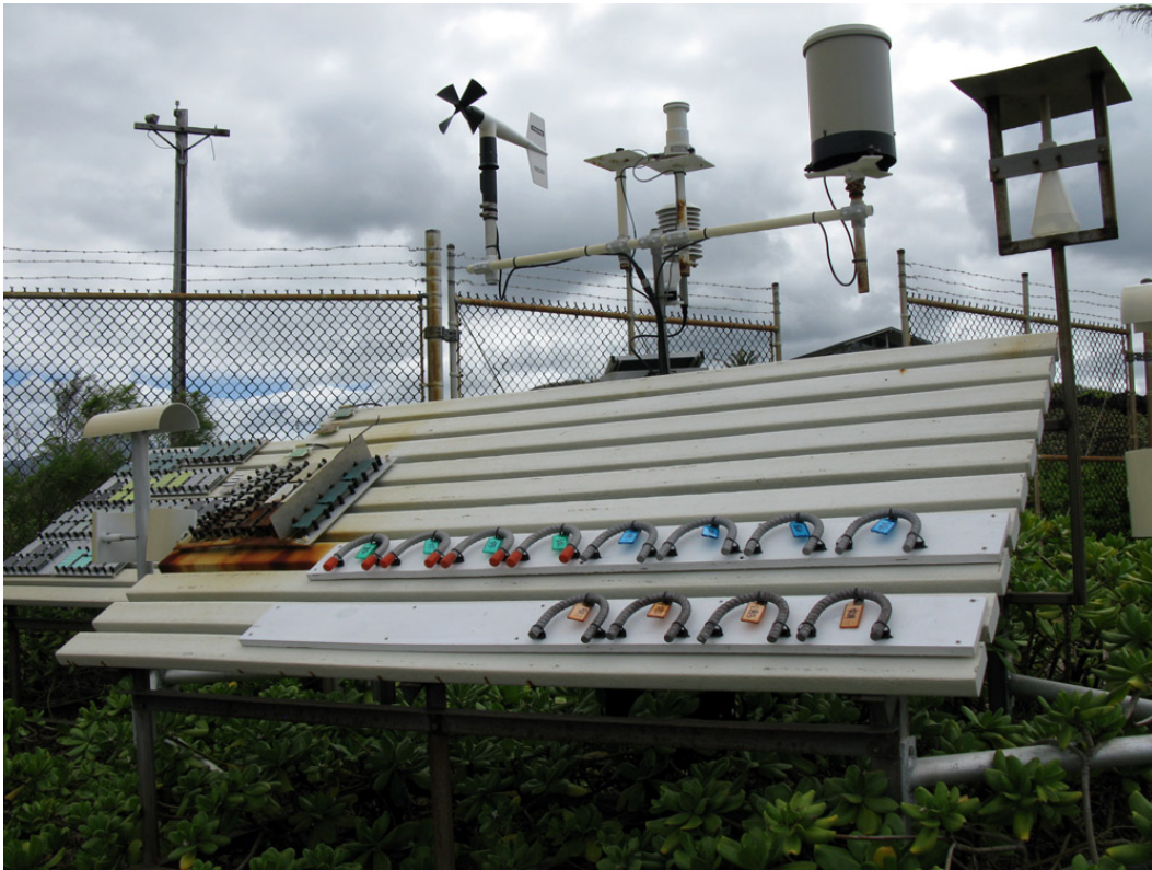
Figure 14. Sample rebar on test rack at MCBH.
