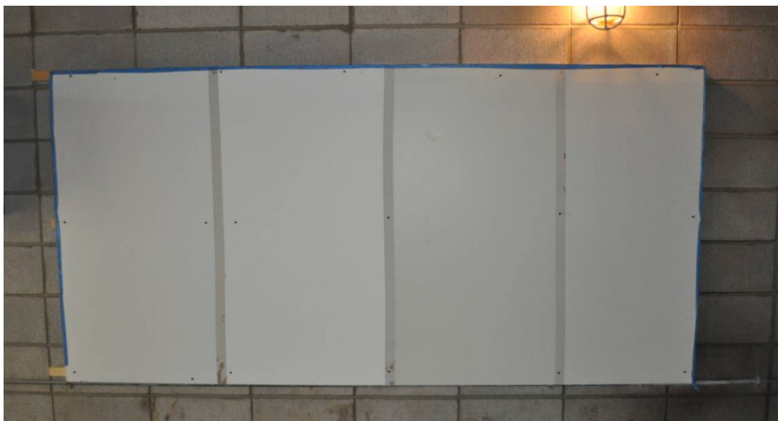
Figure 8. Gypsum board coated with Sherwin Williams ProMar 200, Hirshfield's Platinum Ceramic, Caliwel, and Foster 40-20 (left to right) in 2 x 4 foot sections and hung in the mechanical room of Building 1630.
