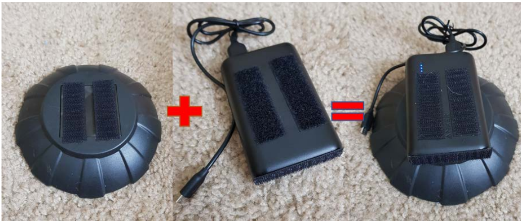
Figure 36. Mounting of Battery Pack onto the Top of Solar Garden Light for Variant B of WGS Node
