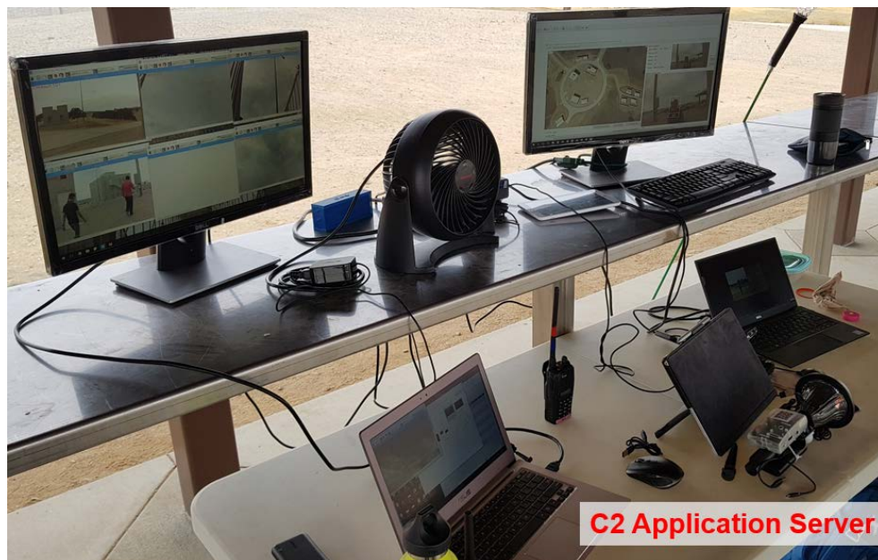
Figure 57. C2 Application Server (right) and Real-Time WGS Node Video Monitoring Station (left) Deployed in the Sheltered Training Shed at CACTF
