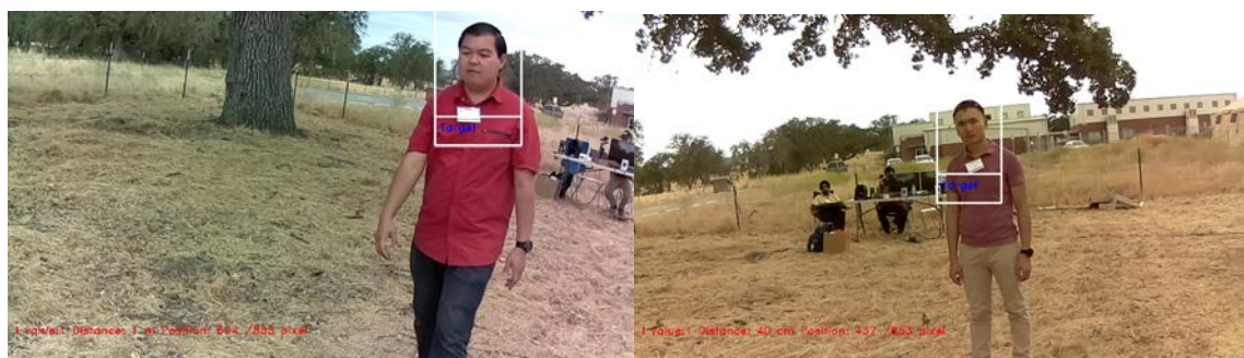
Figure 78. Facial Recognition from RPi_8 (left) and RPi_9 (right) WGS Node at 4m Range
