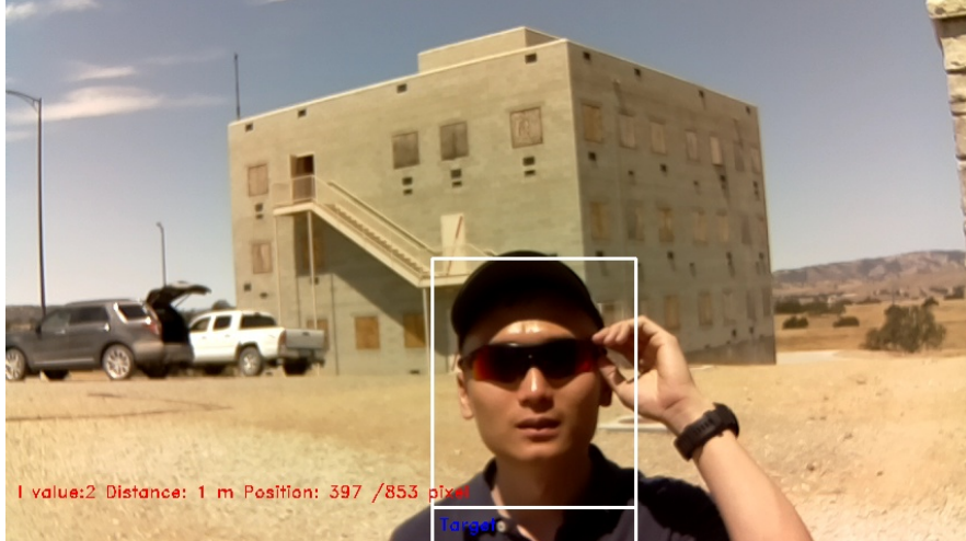
Figure 59. Intruder Wearing Sunglasses and Hat Being Detected by the WGS Node
