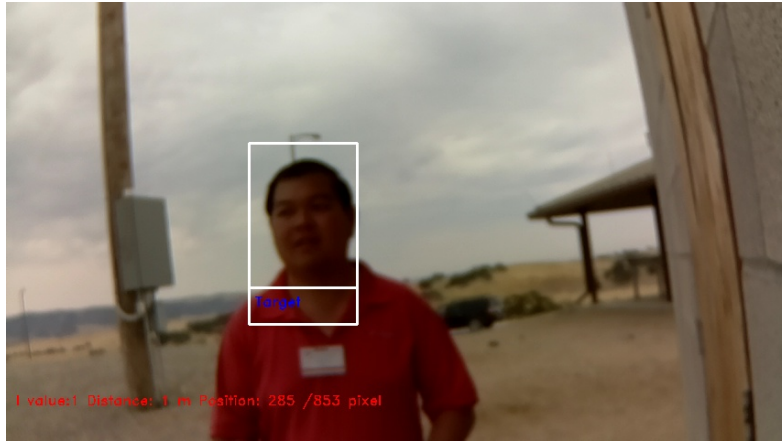
Figure 69. Facial Image Detection Capability of the WGS Node under Low Lighting and Out-of-Focus Condition
