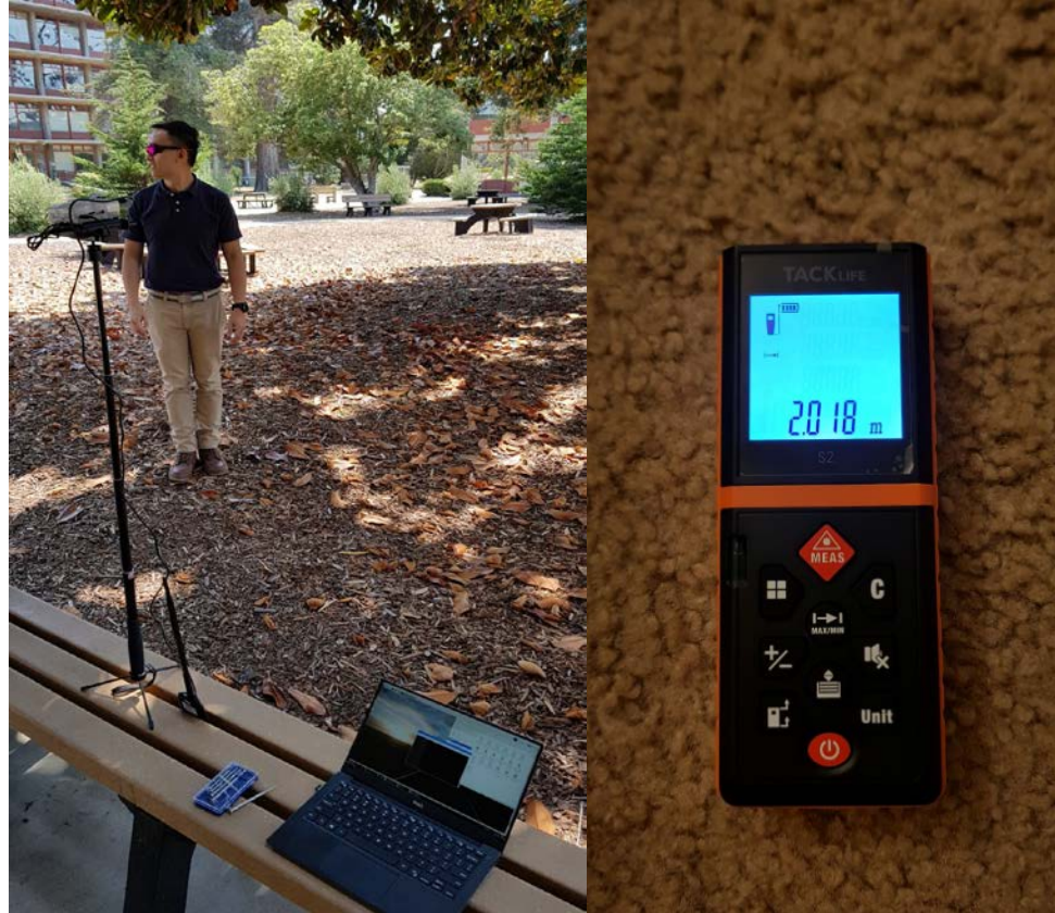
Figure 44. PIR Sensor and Camera Test Setup with Laser Distance Measurement Tool
