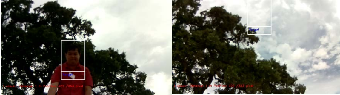
Figure 82. Overcast of Strong Backlight Causing Silhouette Effect and False Positives
