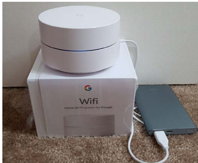
Figure 29. Google WiFi Mesh Router Powered Using Battery Bank
