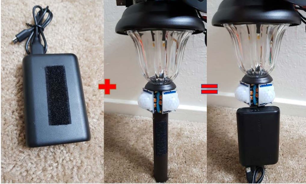
Figure 35. Mounting of Battery Pack onto the Solar Garden Light for Variant A of WGS Node
