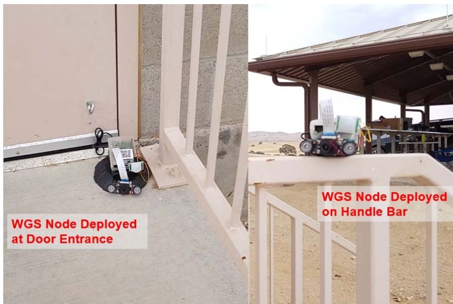
Figure 65. Placement of WGS Nodes at Door Entrance and Stairs Railing around the Two-Level Building
