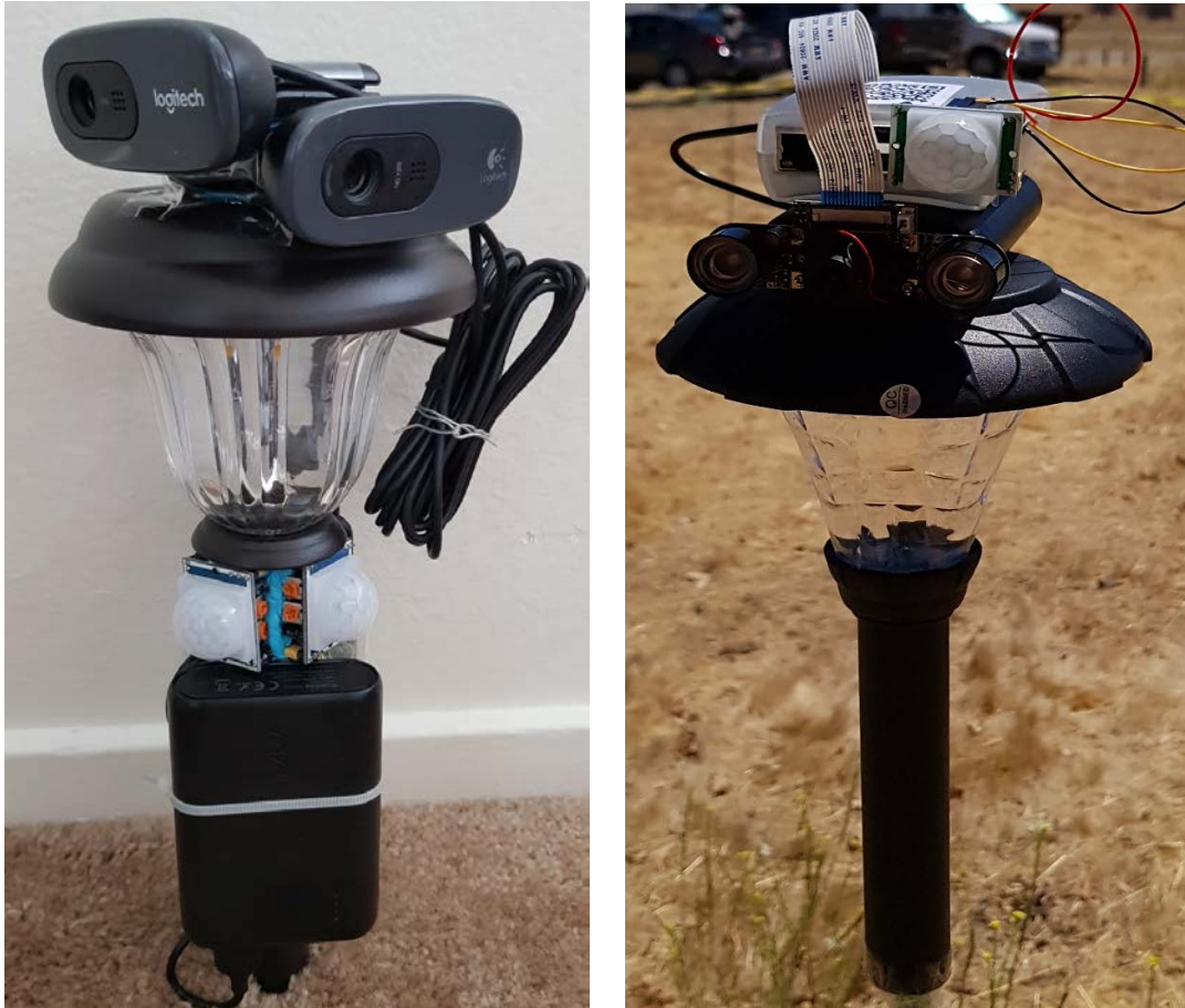
Figure 4. Variant A of WGS Node (left) and Variant B of WGS Node (right)
