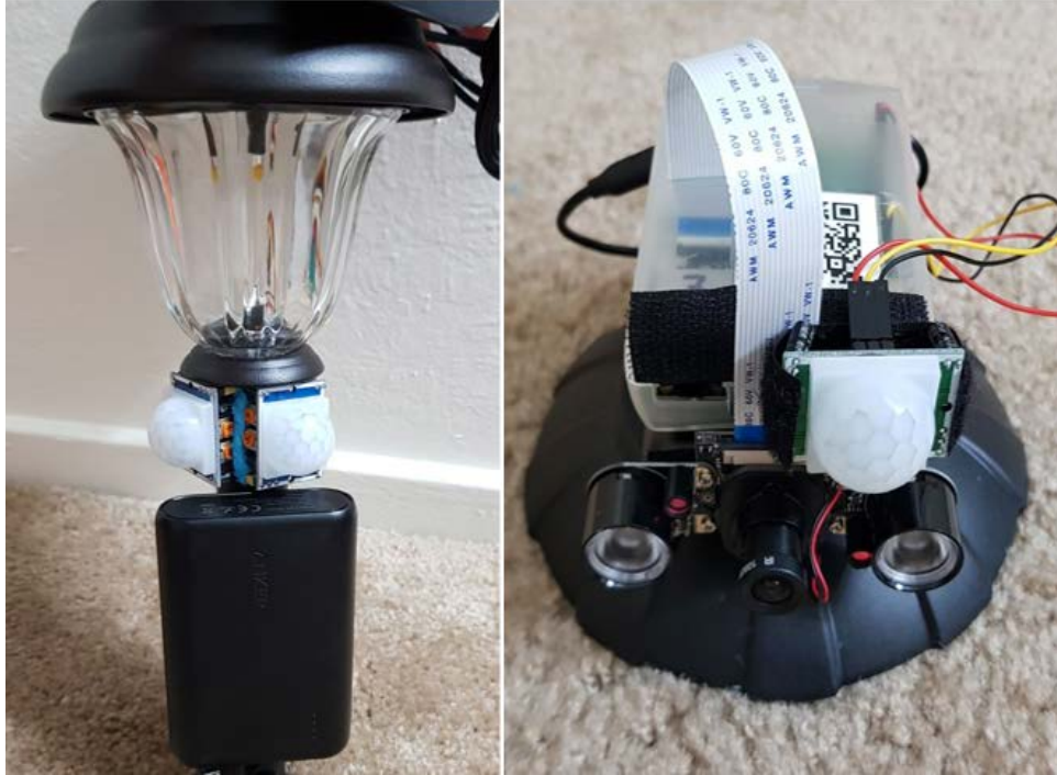
Figure 39. Mounting of PIR Sensor onto the Solar Garden Light for Variant A (left) and Variant B (right) of WGS Node
