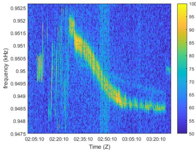
An almost 30-minute compass calibration period can be seen on the left side of the figure. Also, the relatively shallow angle of the frequency change over the central frequency of 950 Hz was not expected based on predicted EMATT tracking relative to the Acousonde.
