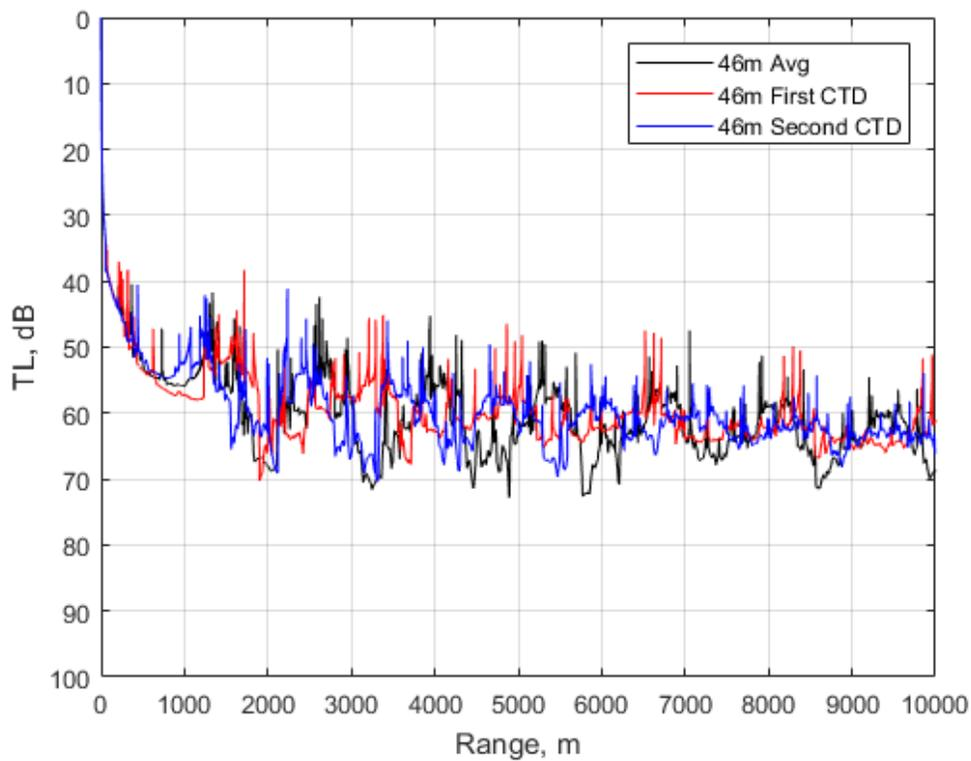
TL using 3 separate sound speed profiles. The red line is the modeled TL for the first CTD at 05:30Z, the blue line is the second CTD at 17:25Z, and the black line is the averaged SSP of both CTDs. This averaged SSP was used to determine the modeled TL in Figures 13–15.
