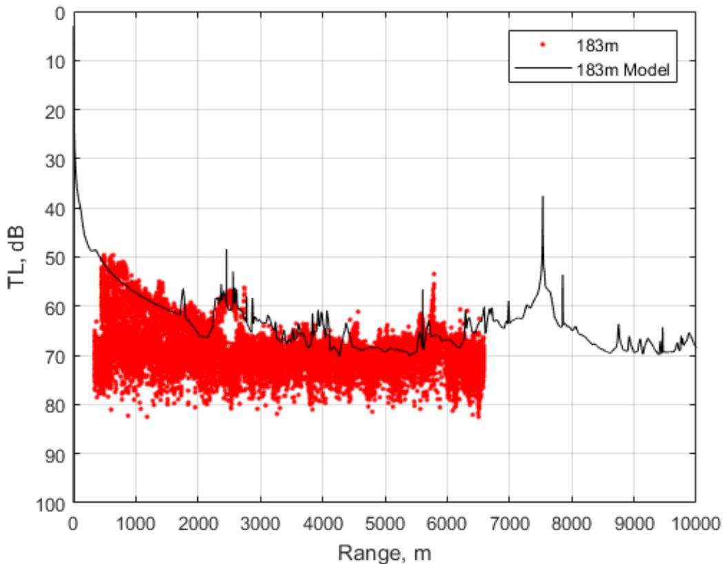
The TL is generally smaller at short ranges, but there are noticeable peaks throughout, specifically at around 2500 meters and 5600 meters for this EMATT/Acousonde combination. Variability is shown to be as high as 30 dB for this frequency. The comparison to the modeled TL shows little in common, other than at short range and both peaks.
