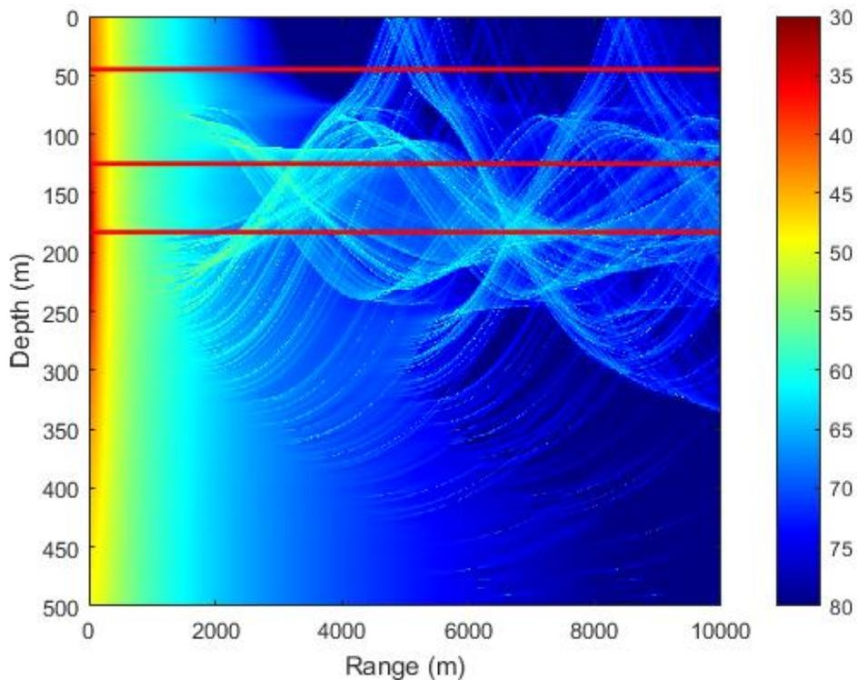
The red lines show the depths at which the Acousonde receivers are. Because the source was mobile, the receivers are represented as lines across range versus point receivers. Strong areas of reception as well as shadow zones can be seen.
