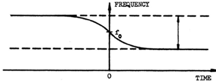
The source frequency is shown as  $f_0$ . The frequency to the left of  $f_0$  is higher, showing the target is approaching the receiver. When the frequency reaches  $f_0$ , the target is at CPA to the receiver. After CPA, the frequency is lower than  $f_0$ , showing the target is moving away from the receiver.
