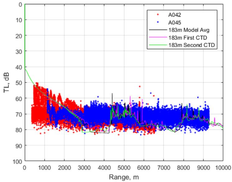
The shadow zones that are present in the modeled data are not present at all in the measured data. For short ranges, the measured TL is less, as is the modeled TL. After about 3000 m, though, the measured becomes flat and does not follow the modeled TL at all.
