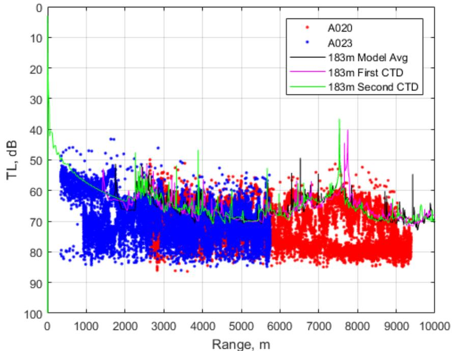
The higher frequency has higher variability, but the general trend of the measured TL follows the modeled TL rather closely, even at further ranges. While the modeled shadow zone at around 5000 m is not present in the measured data, the spikes at 1600 m, 6200 m and even further out at 7500 m can be seen in both modeled and measured data.
