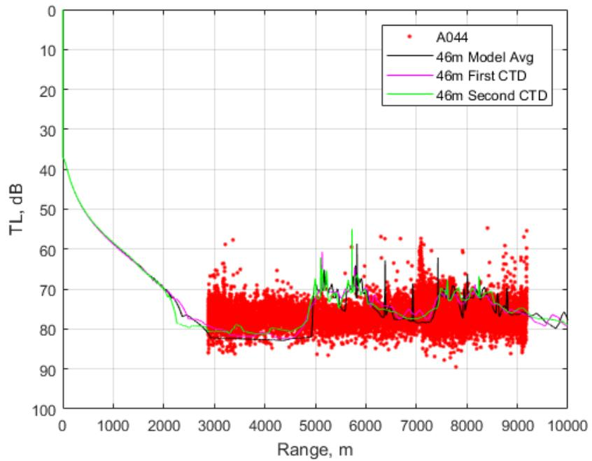
Figure 62. 125m Acousonde (A044), EMATT at 46m, 950 Hz
