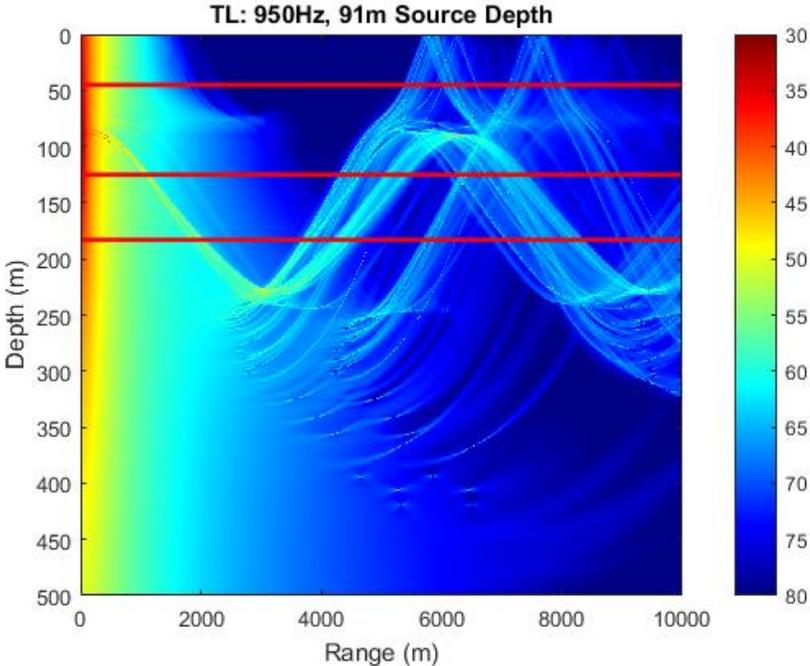
Figure 55. Modeled 950 Hz TL with EMATT at 91m
