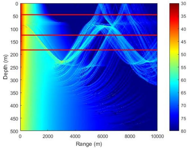
Figure 14. Modeled 2800 Hz TL with EMATT at 91m
