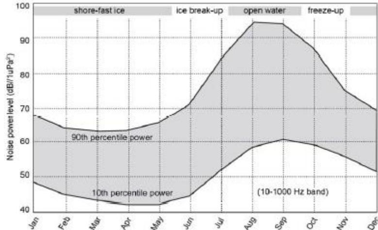
Figure 4. Ambient noise variability due to ice cover in the Arctic.
