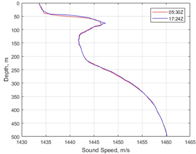
This figure reflects the strong variability around 50-meters depth, and this even extends down to the peak at 80 meters. This variability is temporal and spatial, since the ice (and accompanying CTD measurements) moved throughout the experiment.
