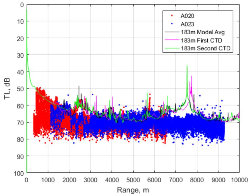
The first area of low TL after 1000 m is at approximately 2300–2700 m. Both the modeled and measured TL follow this trend. Between 4700–5400 m, the modeled TL shows a shadow zone, but the measured TL is actually rather linear. The modeled TL shows a peak in received signal at approximately 7500 m, and this does not show up in the measured TL.
