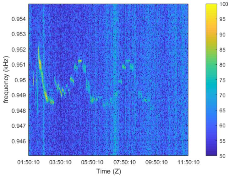
The received frequencies below and above the central frequency of 950 Hz show us the behavior of the EMATT relative to the Acousonde. The Doppler shift is clearly seen as the EMATT travels past the Acousonde early in the run (02:20-03:20), and then circles the Acousonde throughout the next 9 hours.
