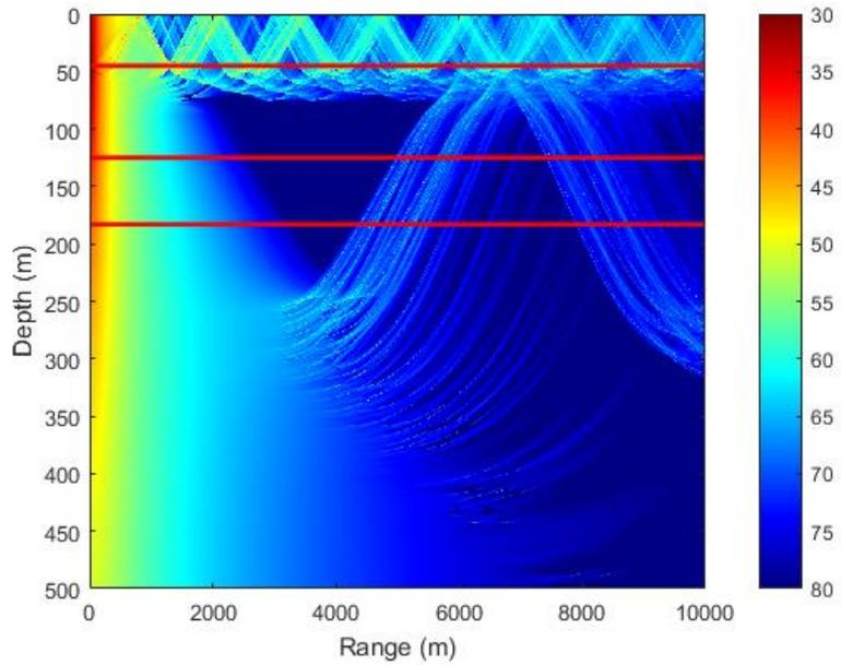
The trapping of sound energy in the surface layer, with the resultant surface interaction, is well demonstrated. Relatively little sound energy is emitted below the layer compared to the other EMATT depths.
