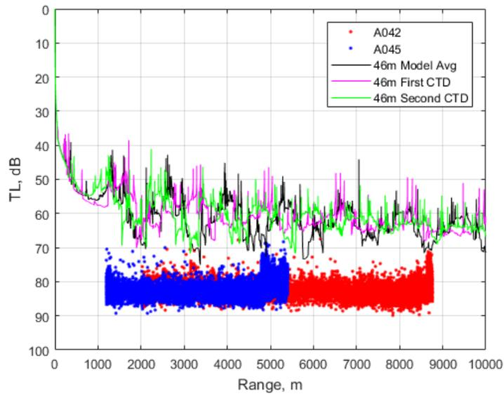
The entirety of the measured TL is very high compared to the modeled TL. In addition, the three modeled TLs (based on the different SSPs) show that the variation over just the 10-hour experiment causes extremely different acoustic paths and highly variable TL.
