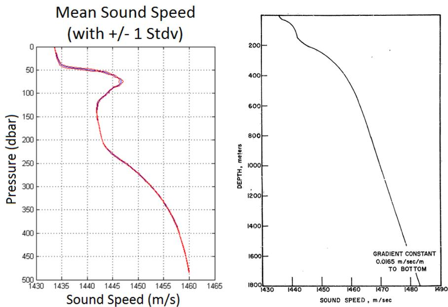
Figure 1. Difference between ICEX SSP (left) and historical Arctic SSP (right).
