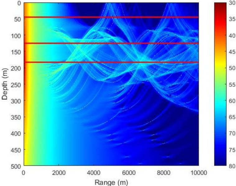
Figure 54. Modeled 950 Hz TL with EMATT at 46m
