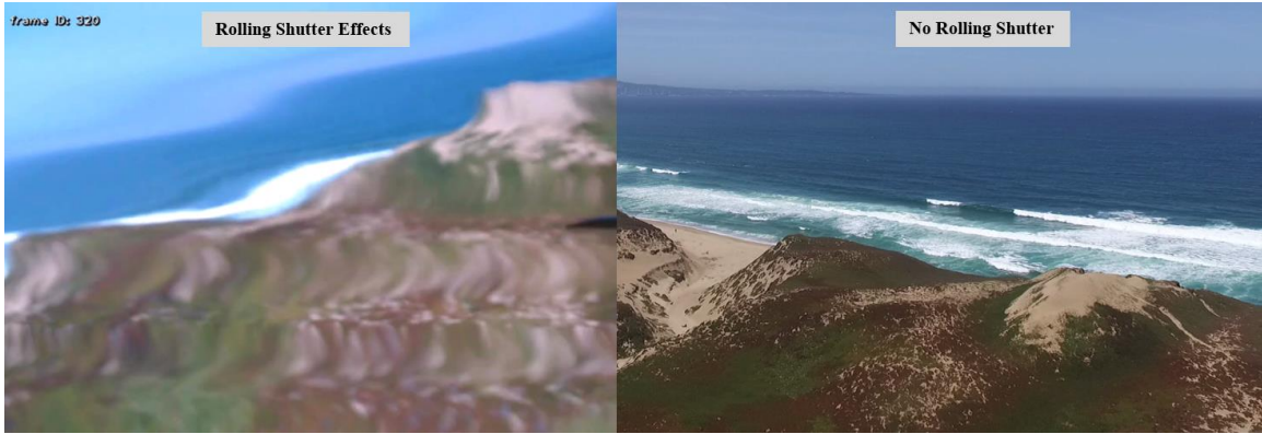
Figure 56. Comparison between Rolling Shutter and Status Quo.
