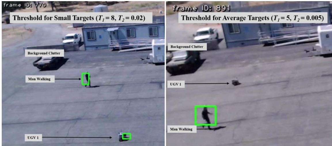
Figure 50. Varying Classifier Parameters at 800 x 600p in Urban Conditions.
