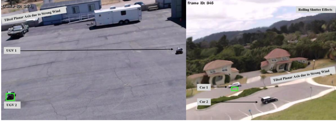
Figure 55. Operation of CV Algorithm in Strong Wind Conditions.
