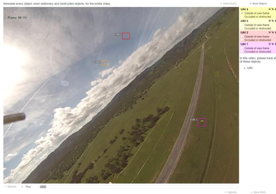
Figure 57. Manual Annotation of Ground-Truth Video Using VATIC.
