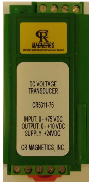
Figure 21 CR Magnetics CR5311-75 DC Voltage Transducer
