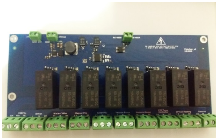
Figure 6. The photo of the 220 V ADC relay board.
