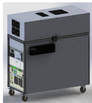
Figure 1. The 3D rendering of the 3 rd generation ^{129}\text{Xe} fully automated stopped-flow hyperpolarizer.
