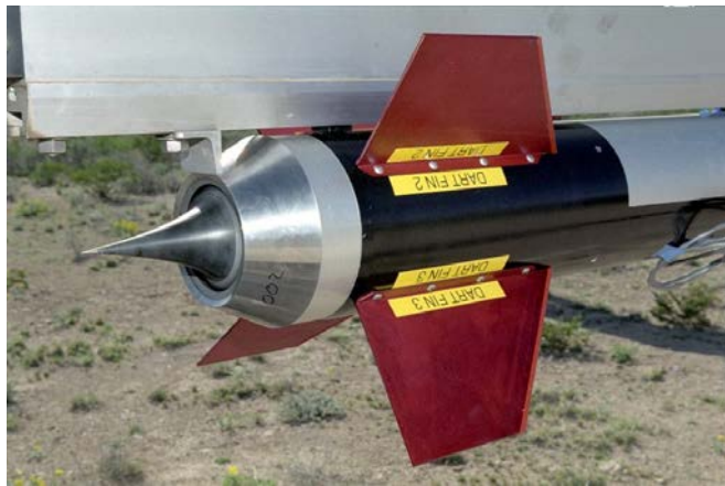
Figure 9. Annular Aerospike Nozzle. Source: [18].
