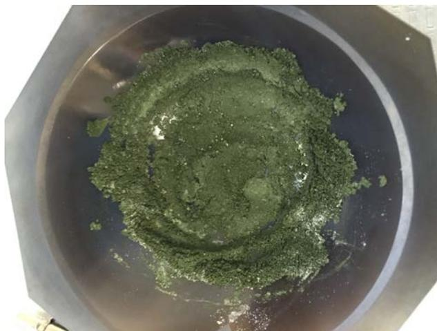
The urea and chromium precursor powders were mixed using the mortar and pestle to create a uniform powder.
