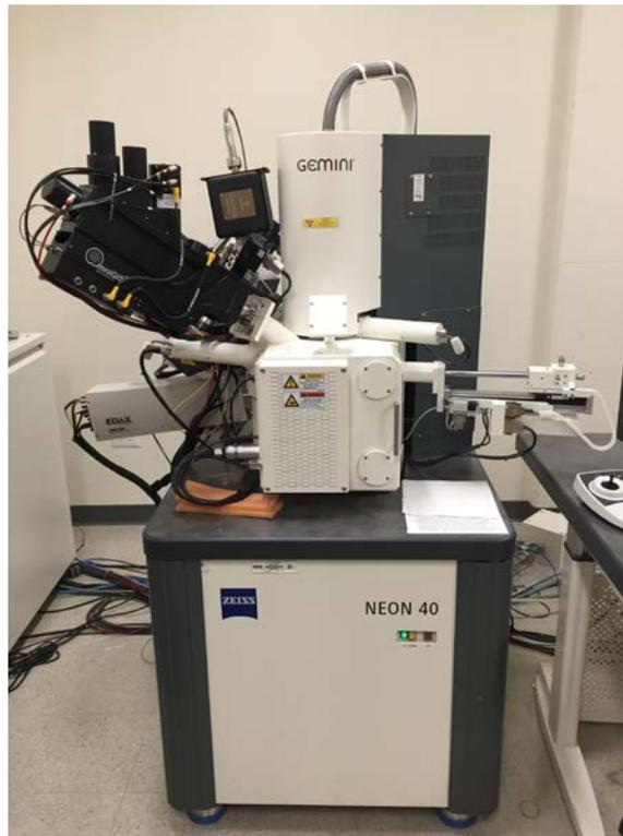
The Zeiss Neon 40 scanning electron microscope was used to characterize the coated samples and powders by using energy dispersive spectroscopy.
