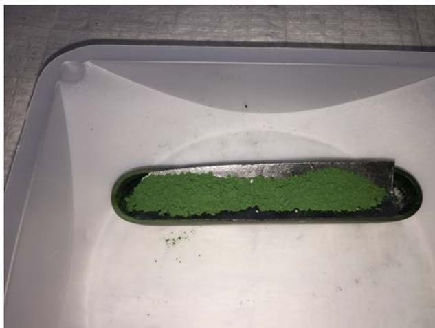
The chromium precursor was placed on top of the graphite foil, which was placed over the lignite and potassium carbonate mixture.
