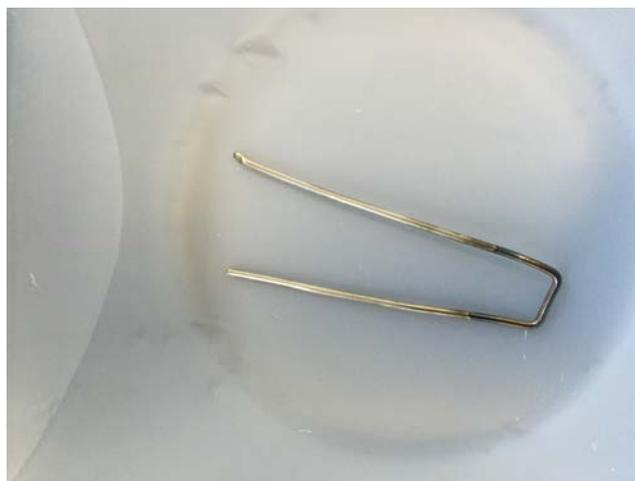
After rinsing and cleaning the coated sample was observed to be very shiny, which led a hypothesis that a thin chromium layer formed on the iron substrate.
