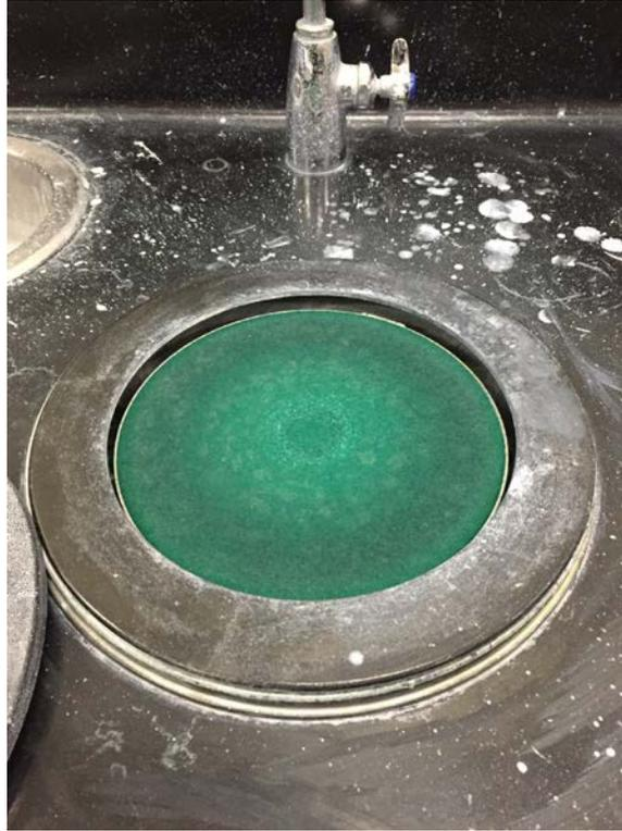
Buehler polishing wheel used to polish sample for 30 minutes.
