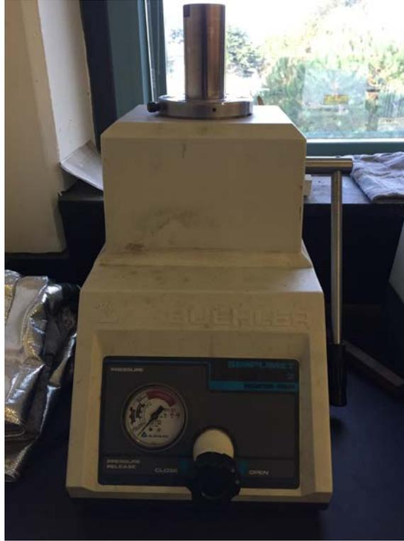
This mounting press was used to mount samples to characterize the cross sections and measure the nominal thickness of the applied coatings.
