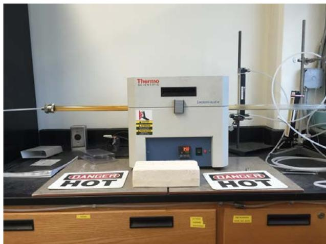
Decomposing chromium nitrate nonahydrate to form the precursor material at 800°C.
