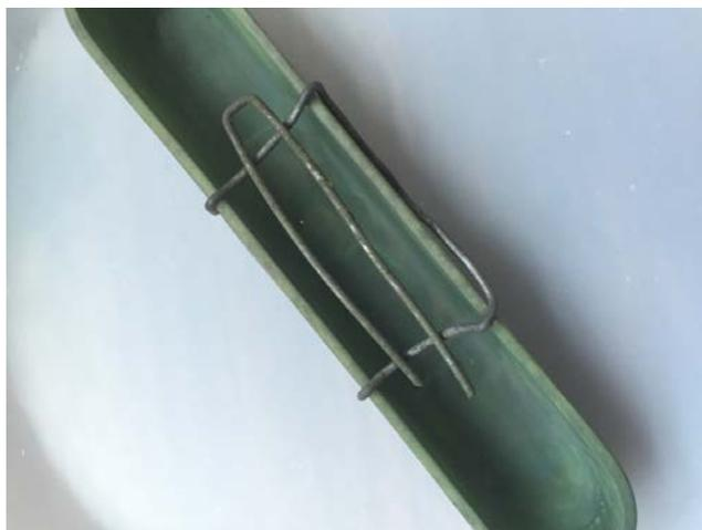
After removing the sample from the quartz tube, it was observed to have a dark green brittle coating.
