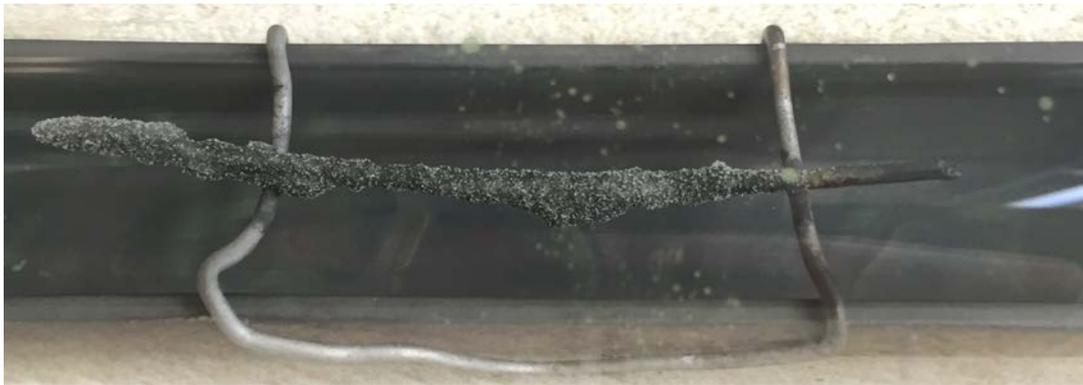
When the coated iron wire paste began to dry, white precipitates began to form on the exterior of the coating.
