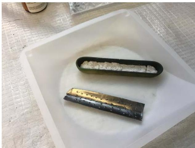
Lignite and potassium carbonate mixture were placed in the crucible with a perforated piece of graphite foil.
