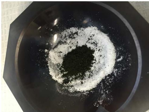
This image shows the chromium based precursor being added to the urea powder for further processing.
