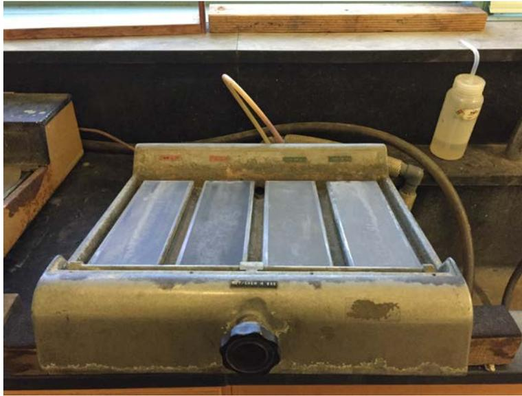
Buehler grinding table used to grind the mounted samples prior to polishing.
