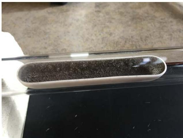
The reduced nickel powder cooling to room temperature.
