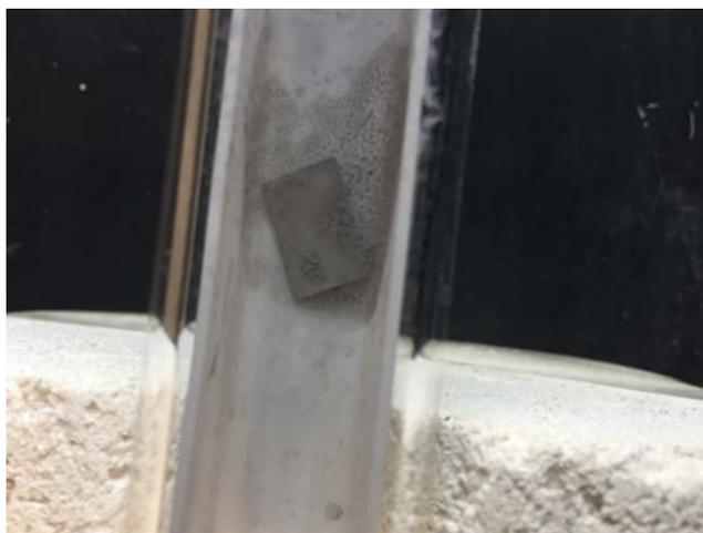
Nickel coated foil sample cooling to room temperature.
