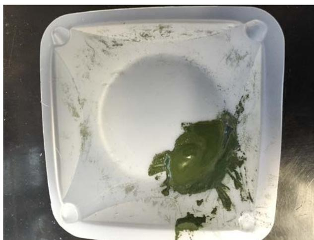
Deionized water was added to the mixed urea and chromium precursor powder to create a paste applied to the iron substrate.
