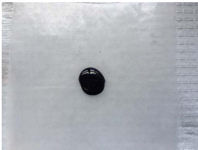
By mixing the urea with the chromium (III) nitrate nonahydrate, it began to form a paste that was then further processed prior to applying to an iron wire sample.
