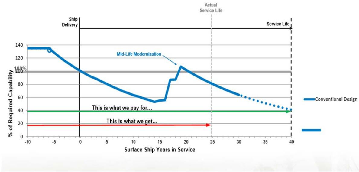
Figure 1. Conventional Surface Combatant Service Life Source: Sturtevant (2015).
