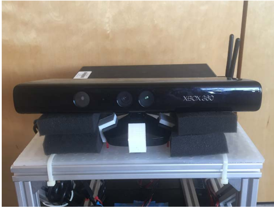
Figure 24. Microsoft Kinect Sensor with Foam Pieces Added for Stability
