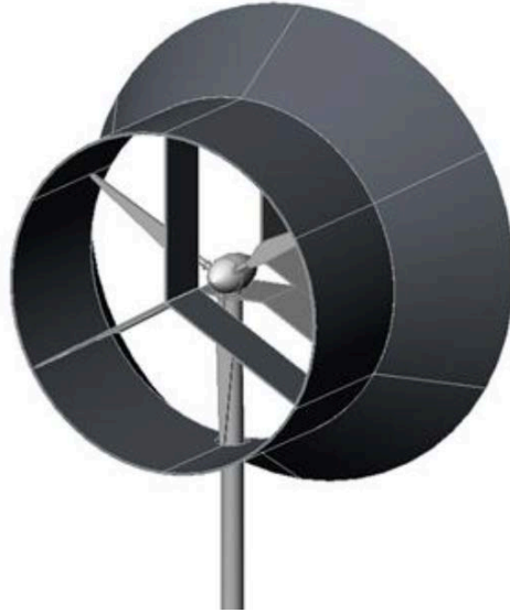
Figure 5. Wind Turbine with Shroud: Preliminary Design. Source: [8].
