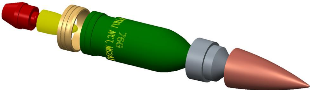
Figure 4 M62A1 APC - exploded view
