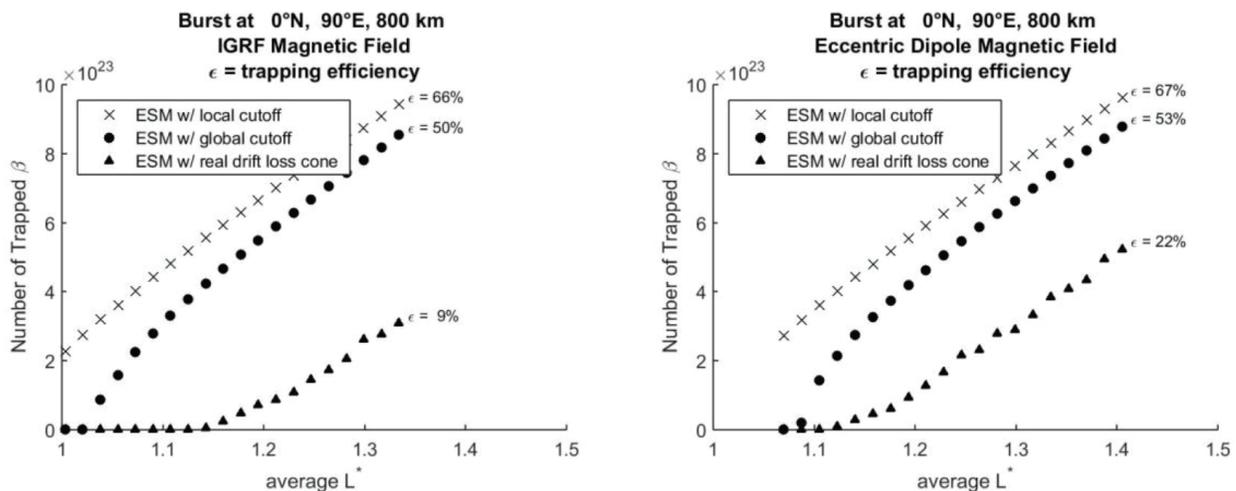
**Figure 3.** Total number of trapped electrons versus  $L^*$  using the eccentric dipole (right) and IGRF (left) magnetic field models, for a burst far from the South Atlantic Anomaly at 800 km altitude. Trapping fractions were computed using a) the local bounce loss cone with 120 km atmosphere (x), b) the local bounce loss cone with 500 km atmosphere (circle), and c) by identifying those electrons that are on closed drift shells (triangles).
