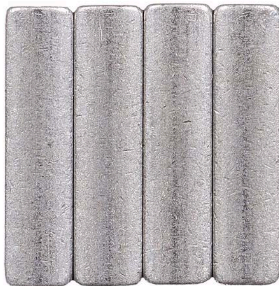
Figure 84. Pump SN:17200858 Transfer Pump Blade Edges before Testing with 30/70 ATJ/F-24 with 24-ppm CI/LI Fuel at 40 °C
