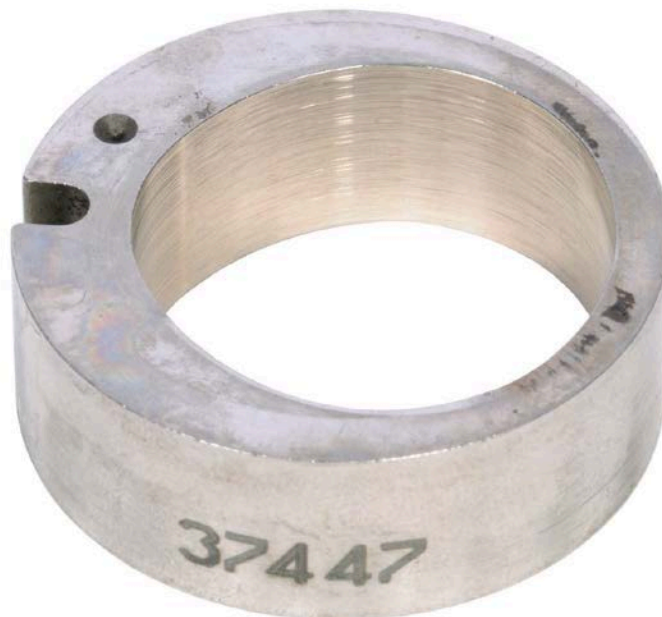
Figure 83. Pump SN:17200858 Transfer Pump Liner with 1000-Hours Testing with 30/70 ATJ/F-24 with 24-ppm CI/LI Fuel at 40 °C
