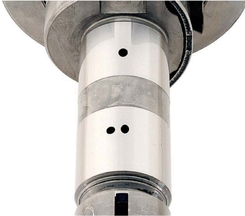
Figure 34. Pump SN:17200045 Distributor Rotor before Testing with 30/70 ATJ/F-24 with 24-ppm CI/LI Fuel at 77 °C
