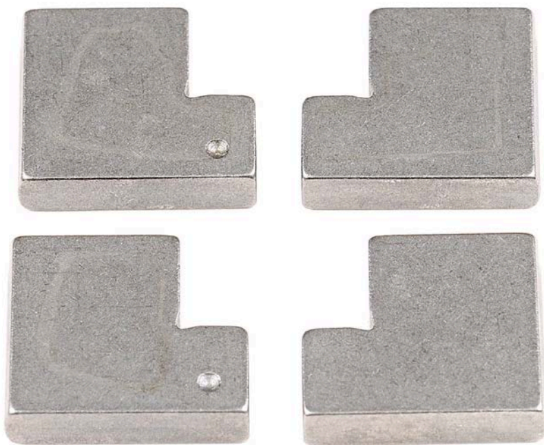
Figure 50. Pump SN:17200045 Transfer Pump Blade Sides before Testing with 30/70 ATJ/F-24 with 24-ppm CI/LI Fuel at 77 °C
