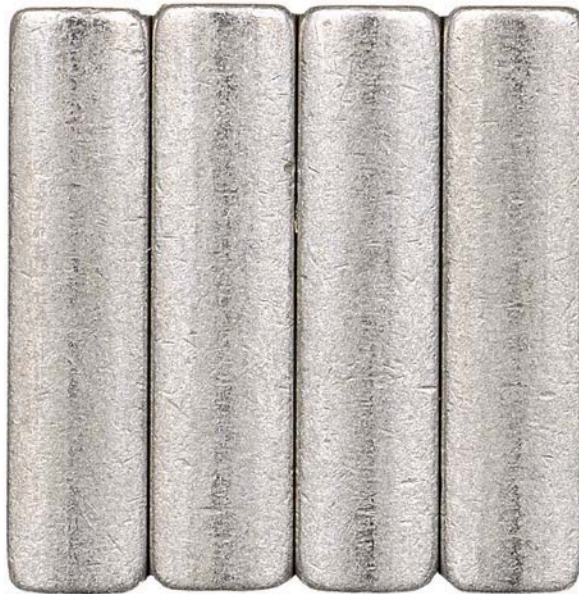
Figure 66. Pump SN:17200072 Transfer Pump Blade Edges before Testing with 30/70 ATJ/F-24 with 24-ppm CI/LI Fuel at 40 °C
