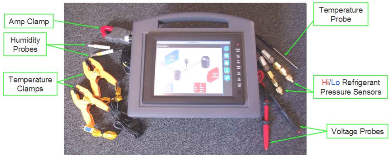
Figure 1. Photo of a Portable i-Optimize Unit, which Incorporates EER Optimizer Technology into a Handheld Diagnostic Tool and Easily Attachable / Detachable Sensors.
