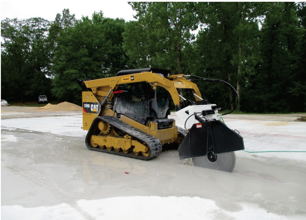
Figure 27. SS3600 diamond blade attachment with a 36-in.-diam blade on a Caterpillar 299D XPS CTL.
