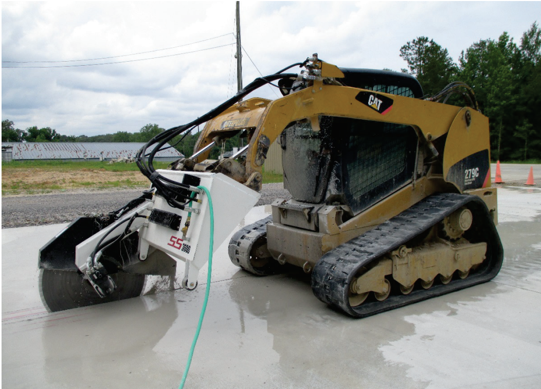
Figure 26. Sludge splattering the windshield of the Caterpillar 279C XPS CTL during cutting.
