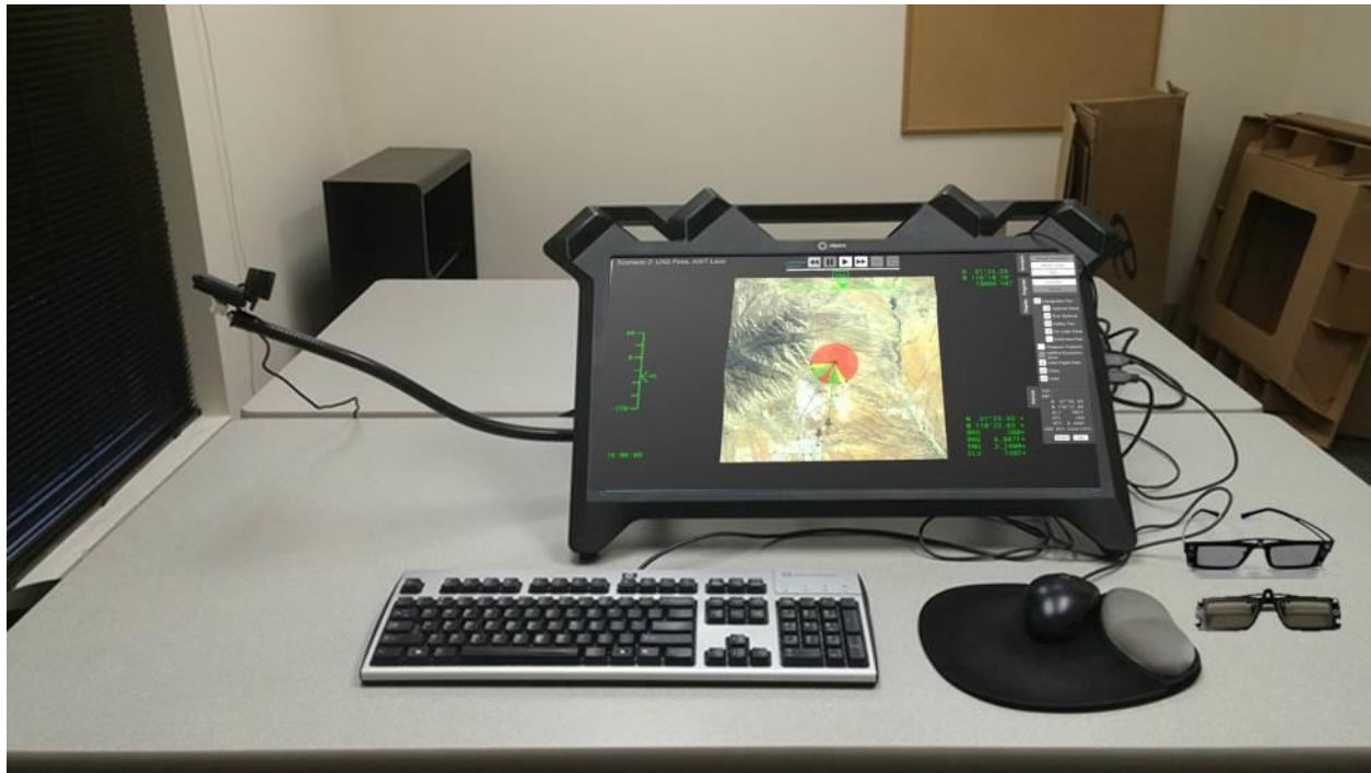
Figure 2. zSpace 200. The zSpace 200 system enables users to view and control graphics in Three-dimensions using polarized eyewear and stylus.
