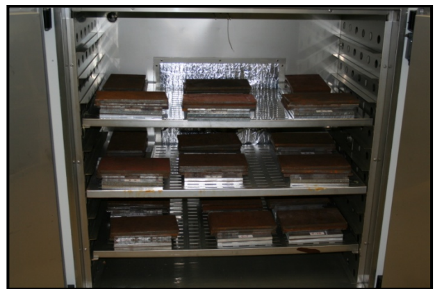
Figure 3. Oven post-curing of single-lap-joints in the bonding tool fixtures.
