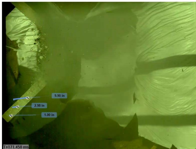
Figure 24. Kinovea applied to a reinforced concrete panel (Test 21).
