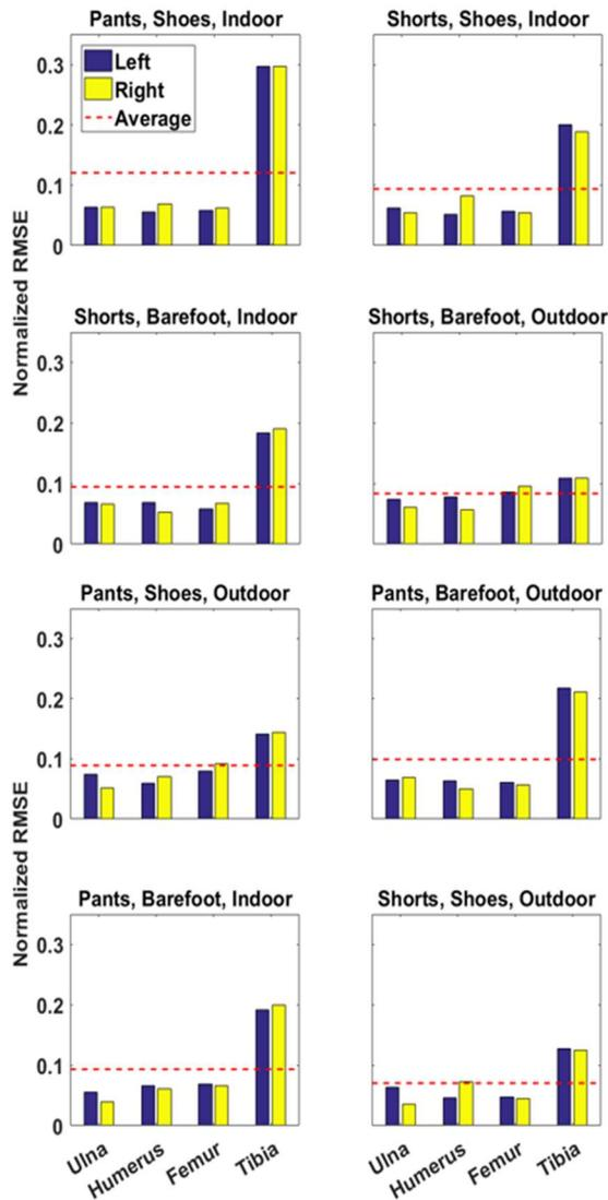
Figure 3: The normalized RMSE for each segment in each condition of the T-pose stance. Blue and yellow bars represent body segment N-RMSE's for left and right side of the body, respectively. The dashed red line represents the overall N-RMSE averaged across all segments.
