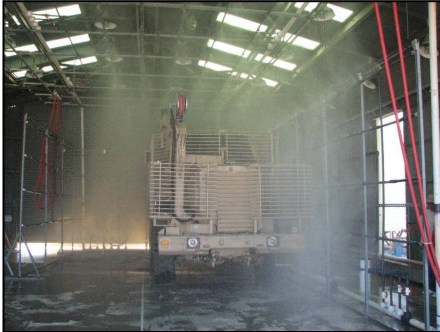
Figure 173. Vehicle inside Rain and Blowing Rain Facility.
