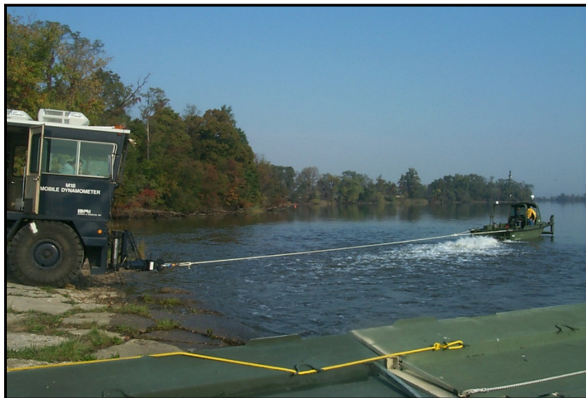
Figure 35. Bollard pull using mobile field dynamometer.
