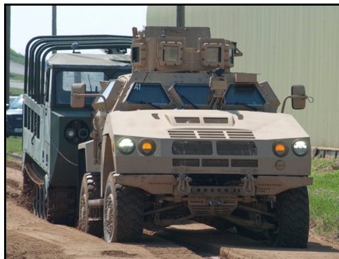
Figure 25. Drawbar pull testing in Sand Course.
