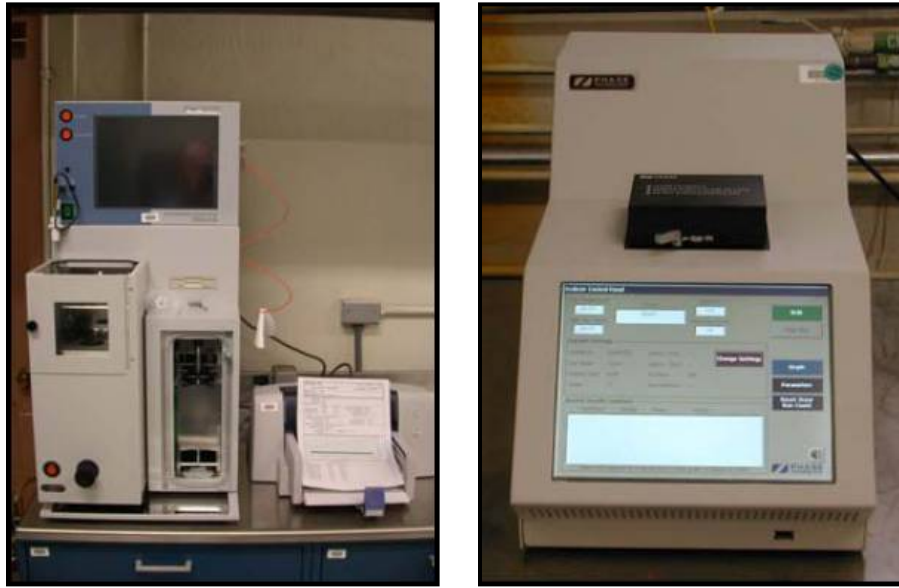
Figure 186. Automatic distillation unit used to measure fuel distillation (left) and automatic cloud and pour point used to measure low temperature characteristics (right).
