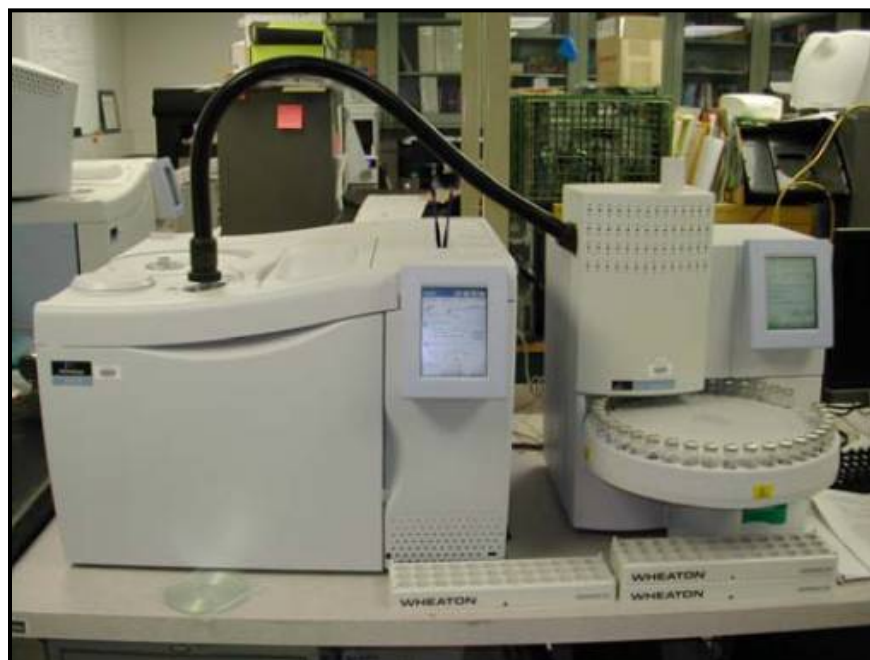
Figure 185. Gas chromatograph with turbomatrix heads pace sampler used to measure diesel fuel dilution.
