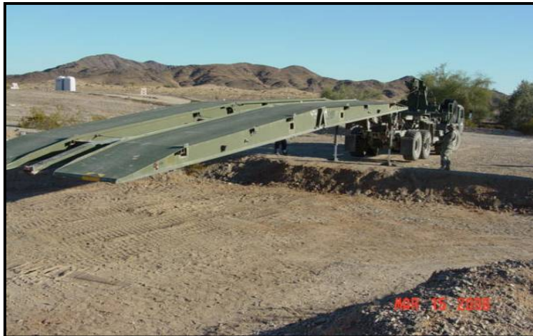
Figure 161. Bridging device test ditch.
