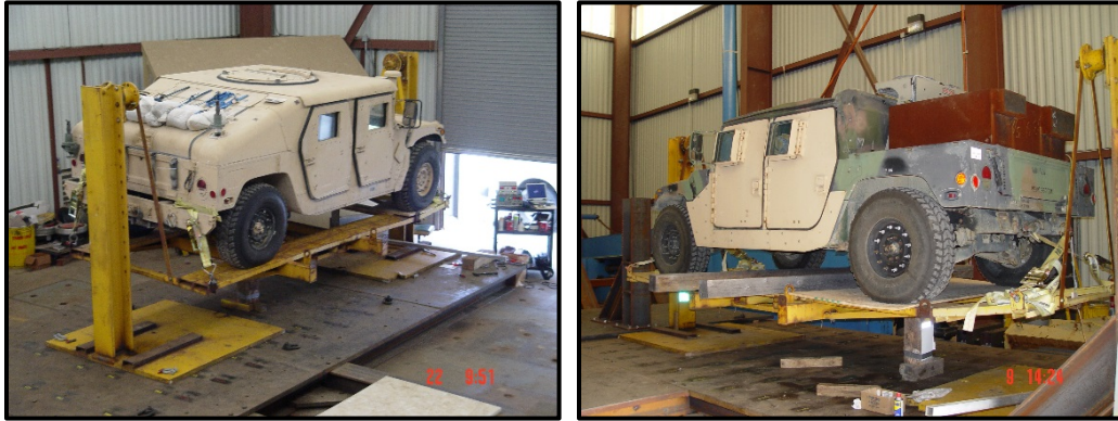
Figure 90. Vehicles subjected to inertia tensor and center of mass testing.
