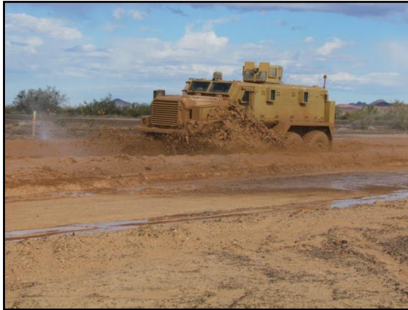
Figure 132. Vehicle operating on Dyno Mud.
