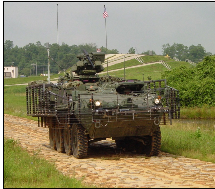
Figure 40. Endurance testing using Imbedded Rock Course.
