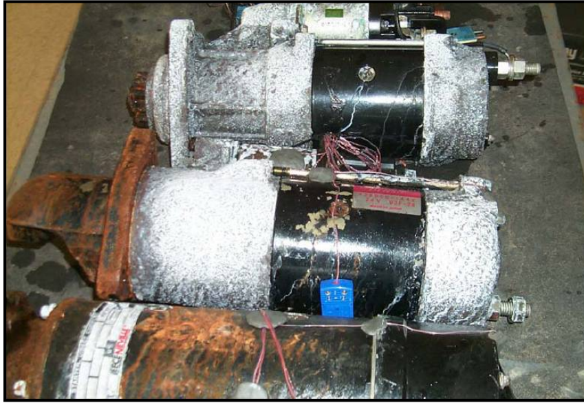
Figure 181. Test item after climatic salt fog testing.
