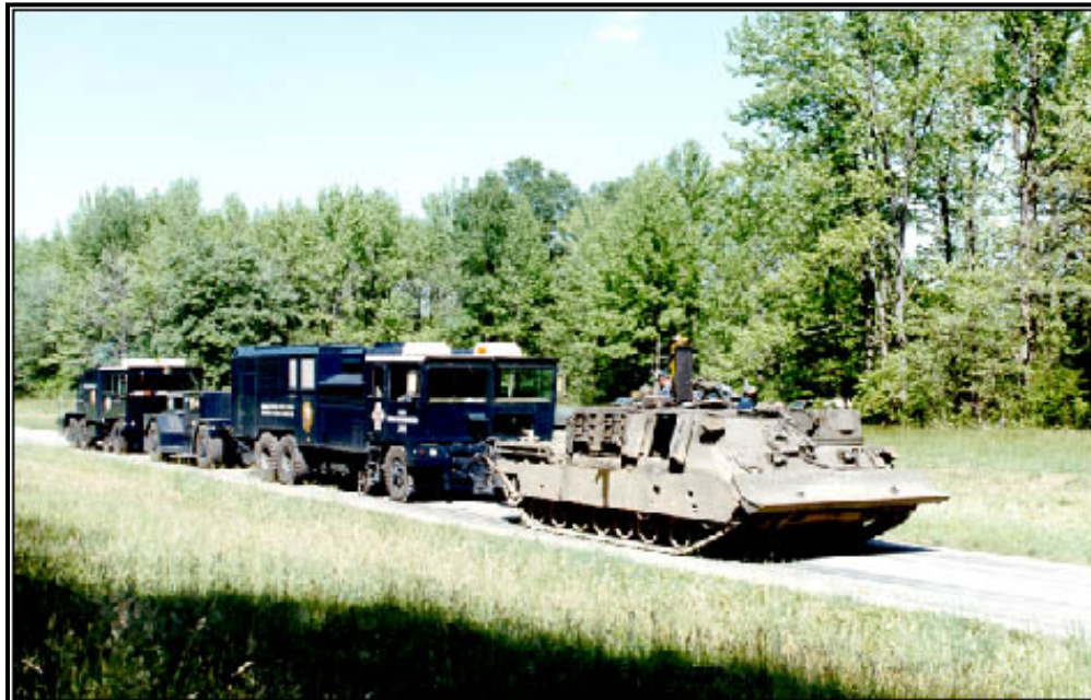
Figure 12. Drawbar pull test conducted on Dynamometer Course.
