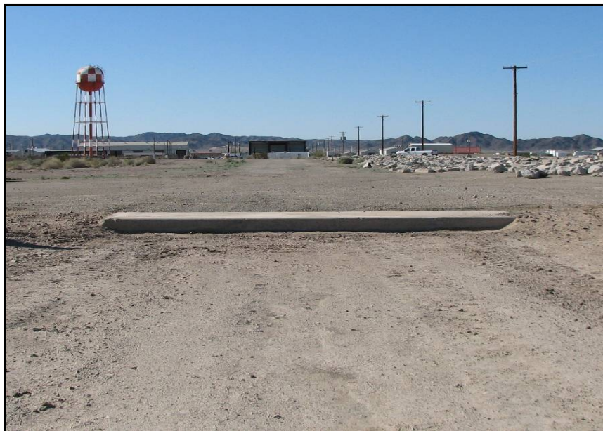
Figure 139. Curb Impact Course.
