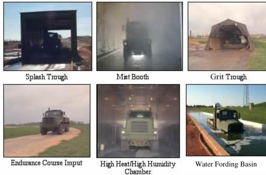
Figure 27. Accelerated Corrosion Complex.
