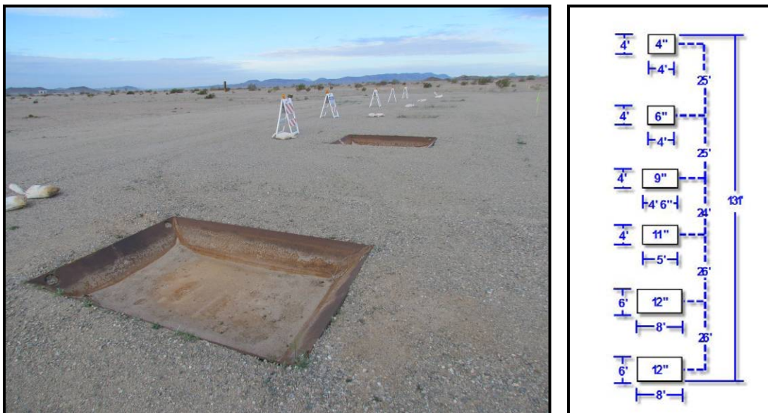
Figure 146. YTC Potholes Course (left) and dimensions of the YTC Potholes Course (right).
