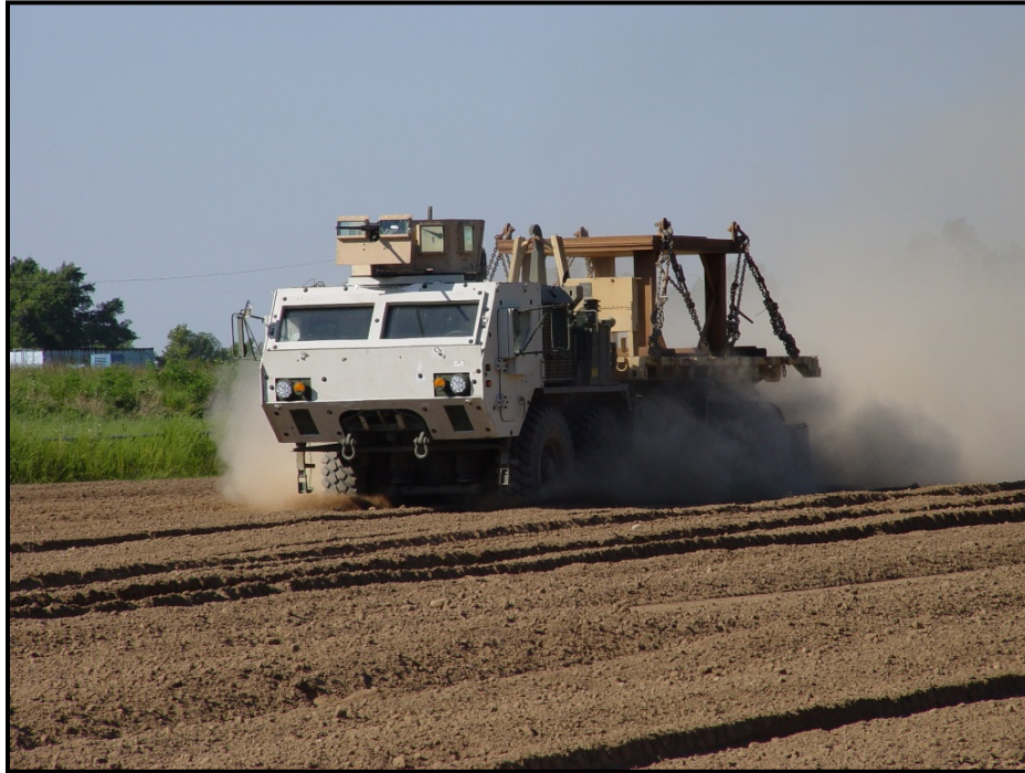
Figure 29. Crossing velocity test in the hog wallow.
