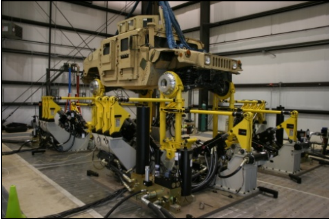
Figure 87. Vehicle Durability Simulator.
