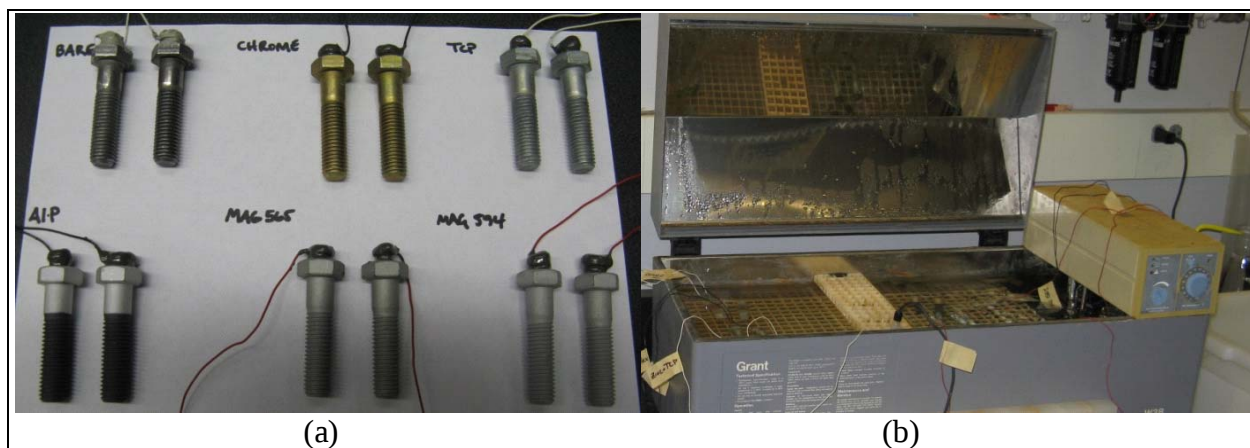
Figure 2. (a) Prepared bolts prior to immersion and (b) immersion bath setup.
