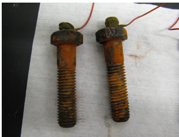
Figure 15. Bare bolts immediately after immersion in supplementary experiment.
