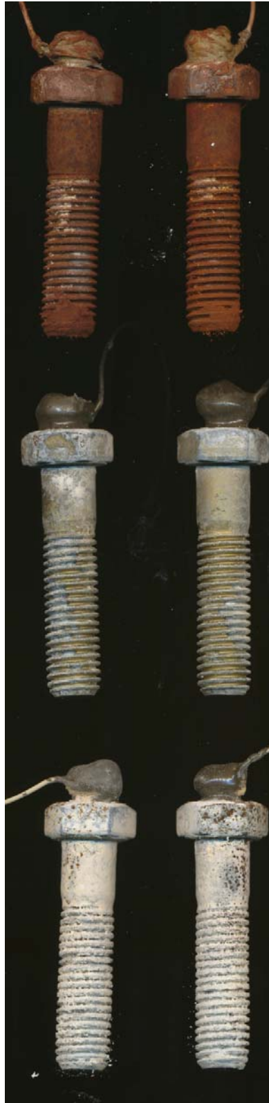
Figure 11. Bare steel, hexavalent chrome/zinc, and TCP/zinc after drying.
