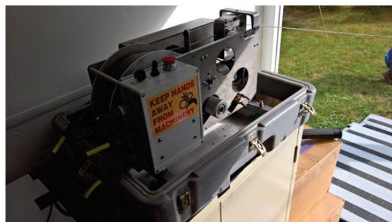
Winch and Data Logger Setup
