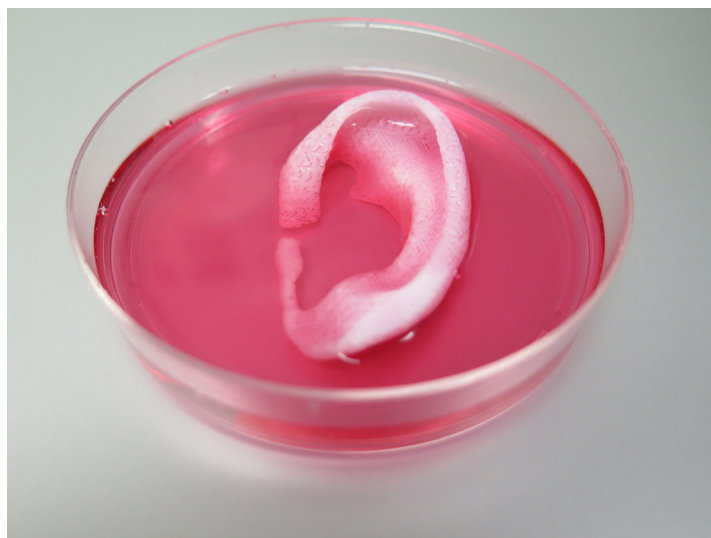
Complete ear structure made using a 3D bioprinter. Source: Wake Forest Baptist Medical Center.
