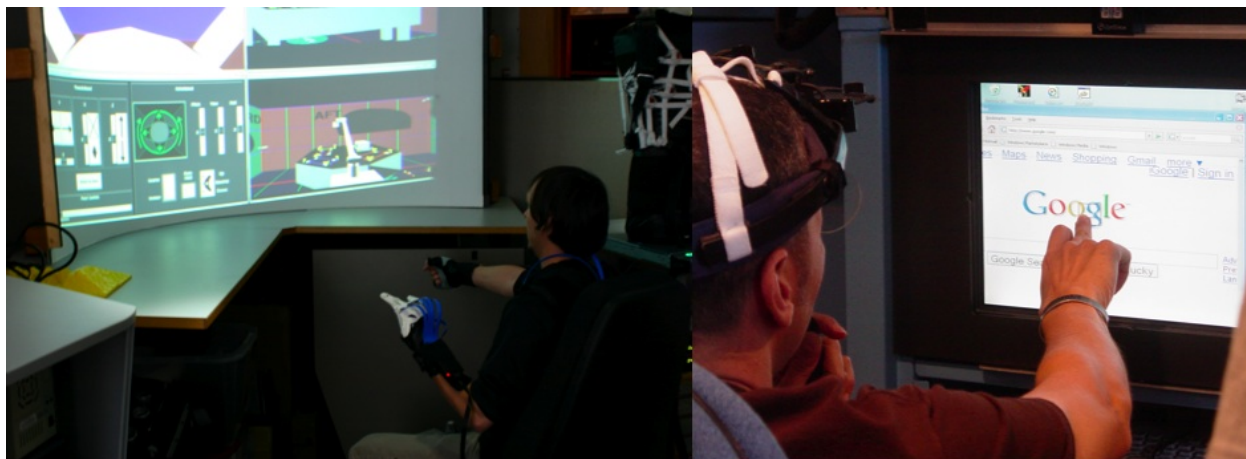
Figure 5: (left) Gesture based controller for robotic arm simulator. (right) Status post binocular enucleation, a servicemember uses his prosthetic eyes to control a tracking reticle on the screen with tactile (tongue based) display of area displayed inside the reticle (near user's finger).
